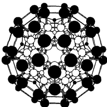
Fig. 1 Geometric structure of Si<sub>60</sub>-coated C<sub>60</sub>. The open and closed circles represent C and Si atoms, respectively.
