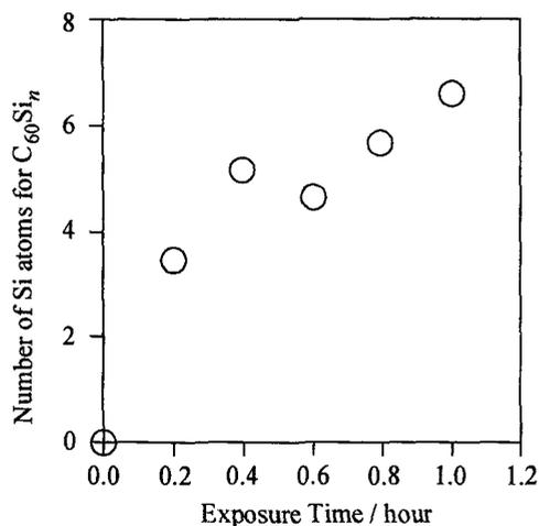
Fig. 3 Number  $n$  of Si atoms for the charge-transfer complex C<sub>60</sub>Si <sub>$n$</sub>  is plotted as a function of exposure time for the Si-atom beam.
