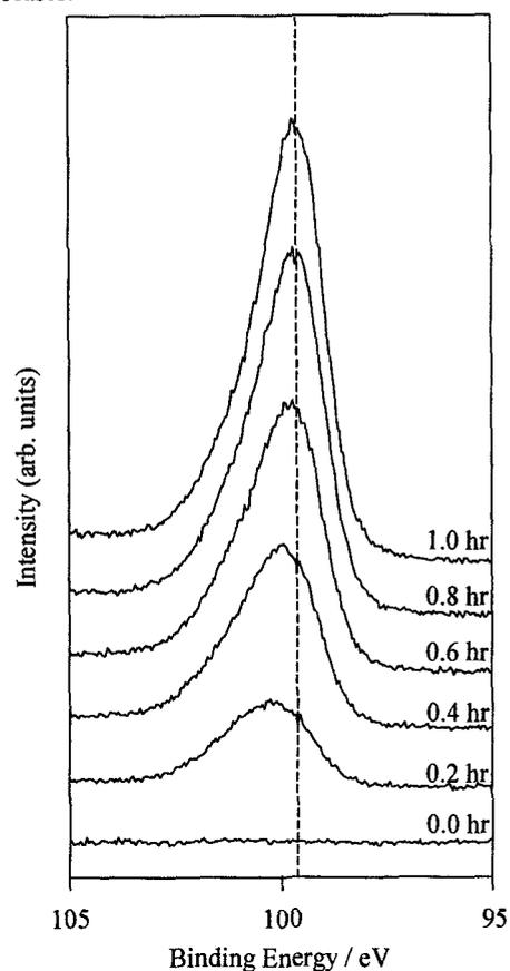
Fig. 2 The Si 2p spectra of Si-deposited C<sub>60</sub> thin film. Total exposure time of the Si-atom beam is represented on the right side of the spectrum, respectively. The dotted line represents a peak position for a clean Si surface.
