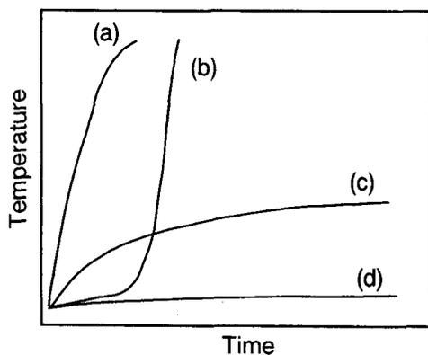
Fig. 2 Typical temperature-time profiles of materials during microwave irradiation. Curves (a) and (b) show strong microwave-material coupling, (c) moderate, and (d) weak.
