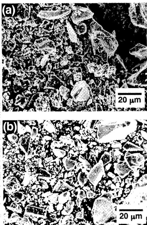
Fig. 6 SEM photographs of (a) starting  $\beta$ -B powder and (b) microwave-processed Fe-doped  $\beta$ -B.
