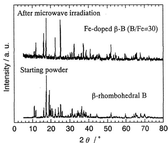
Fig. 5 X-ray diffraction patterns of  $\beta$ -rhombohedral boron and Fe-doped  $\beta$ -boron (B/Fe=30) synthesized by microwave irradiation.
