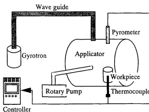
Fig. 1 General scheme of the multimode 28 GHz microwave processing equipment.
