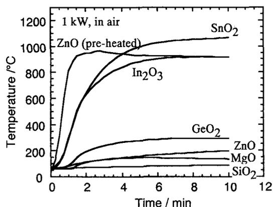
Fig. 3 Temperature-time profiles of p-block oxides during 28 GHz microwave irradiation.
