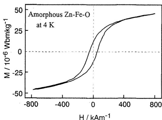
Fig. 4 Magnetic field dependence of magnetization of amorphous Zn-Fe oxide obtained by microwave irradiation.
