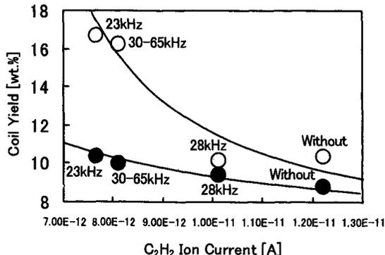
Fig. 2. Effects of the amount of undecomposed acetylene on the coil yield. (○) reaction tube with eight source gas inlets, (●) reaction tube with single source gas inlet.
