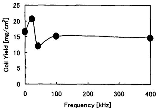
Fig. 1. Effects of the frequency on the coil yield. 0 kHz indicates without irradiation.
