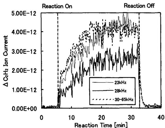
Fig. 3. Effects of the ultrasonic wave irradiation on the amount of decomposed acetylene.
