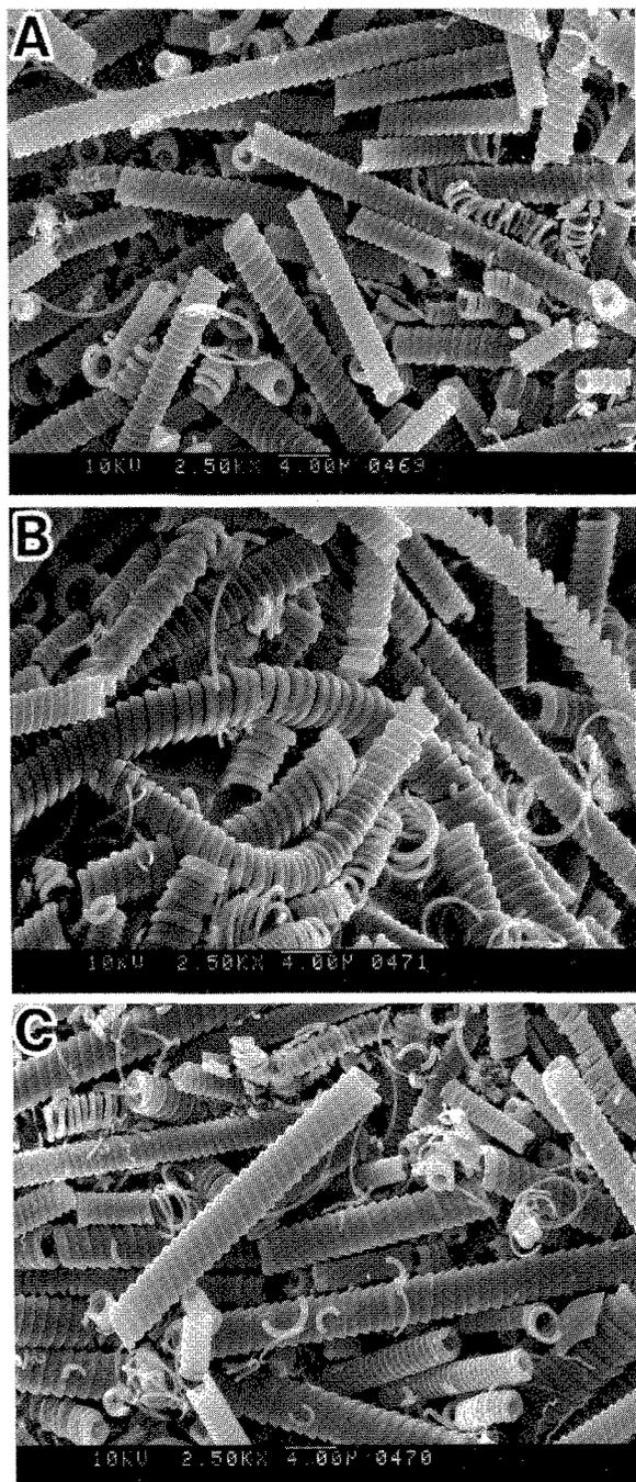
Fig. 4. Representative SEM image of the carbon coils. (a) Without irradiation of ultrasonic waves, (b) with irradiation (23kHz), (c) with irradiation (100 kHz).
