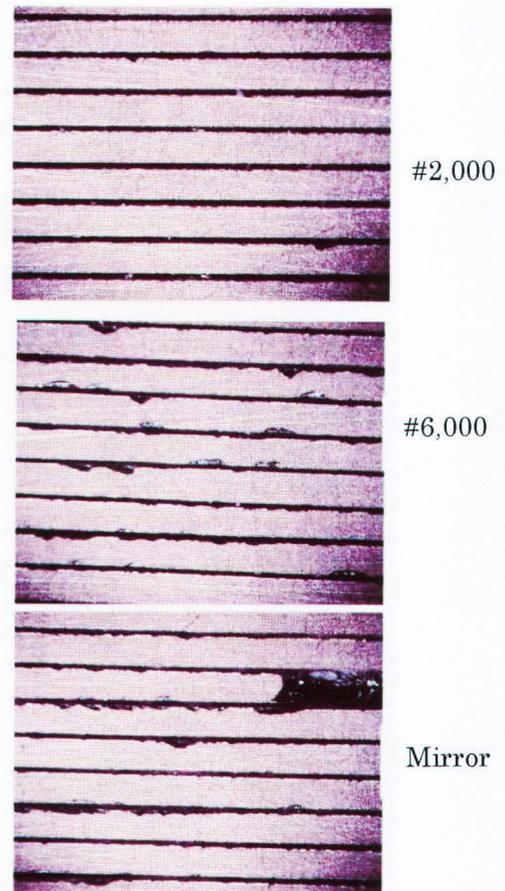
Figure 5. Diced PSC surfaces of different surface conditions, #2,000, #6,000 and mirror lapping (View from the top). Note: Mirror lapping and #6,000 lapped PSC show electrode peeling off and many chipping after dicing. Dicing pitch is 180 micron with 30 micron blade.
