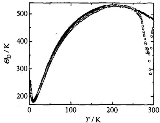
Fig. 4. Debye temperatures of PST and PMN single crystals calculated from the measured heat capacities assuming  $15N_A$  degrees of freedom. ○: PST, ●: PMN.
