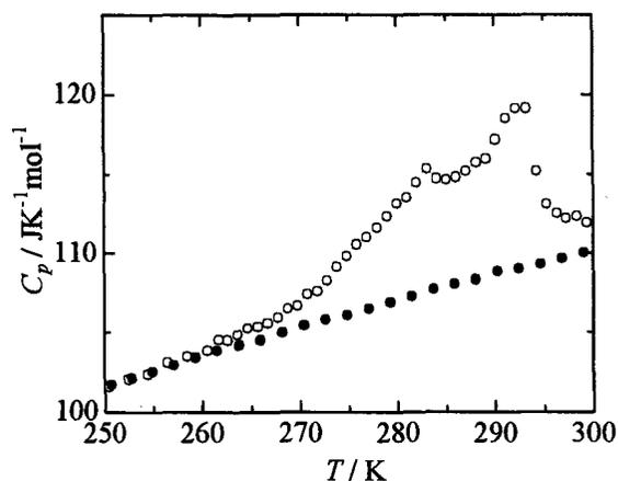
Fig. 2. Heat capacity of PST and PMN single crystals near the ferroelectric phase transition of PST.  $\circ$ : PST,  $\bullet$ : PMN
