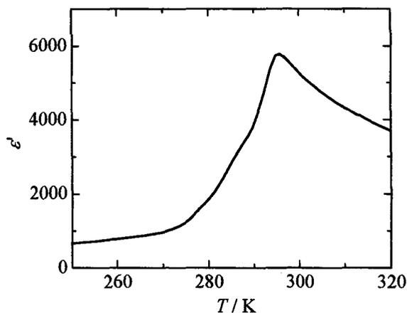
Fig. 3. Dielectric constant of PST single crystal near the ferroelectric phase transition temperature.
