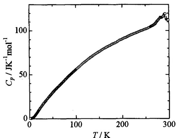
Fig. 1. Measured molar heat capacity of PST single crystal.
