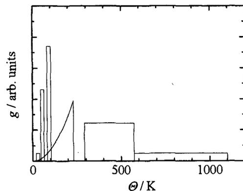
Fig. 6. Density of states of lattice vibrations in PST obtained by fitting to the measured heat capacity.
