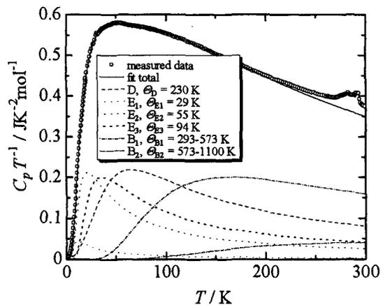
Fig. 5. Molar heat capacity of PST. The solid line is the result of the fitting, and the dashed line and others denote the individual contributions.
