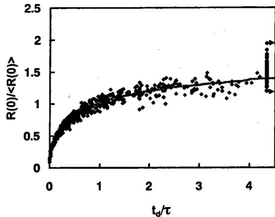
Fig. 4 Plot of life span against initial grain size.
