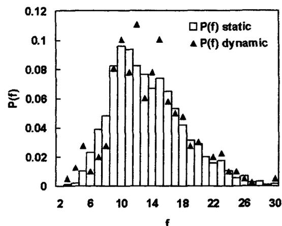
Fig. 9 Distribution function of the number of faces in the steady structure (static) and that from the dynamic analysis.
