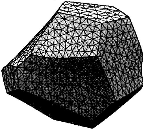
Fig. 2. Example of triangular mesh of a grain
