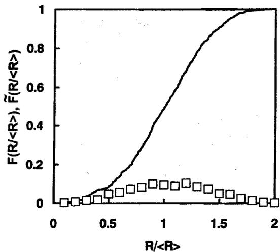
Fig. 5 The distribution function ( $\square$ ) and the cumulative distribution function (solid line) in normal grain growth.
