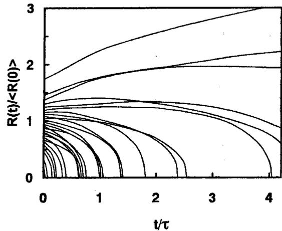
Fig. 3 Variation in the individual grain size with time in normal grain growth. The curves for some selected grains are shown.
