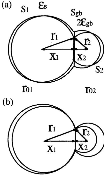
Fig.1 Models for sintering(a) and grain growth(b). Two spherical grains with different size of radii  $r_{01}$  and  $r_{02}$  ( $r_{01} \geq r_{02}$ ), initially (time  $t=0$ ) in contact at a point, join together after time  $t$  forming the grain boundary.  $r_1$  and  $r_2$  are the radii of grains 1 and 2,  $x_1$  and  $x_2$  are the distances between the grain centers and the boundary,  $S_1$ ,  $S_2$  and  $S_{gb}$  are the surfaces of grains 1, 2 and the boundary, respectively.
