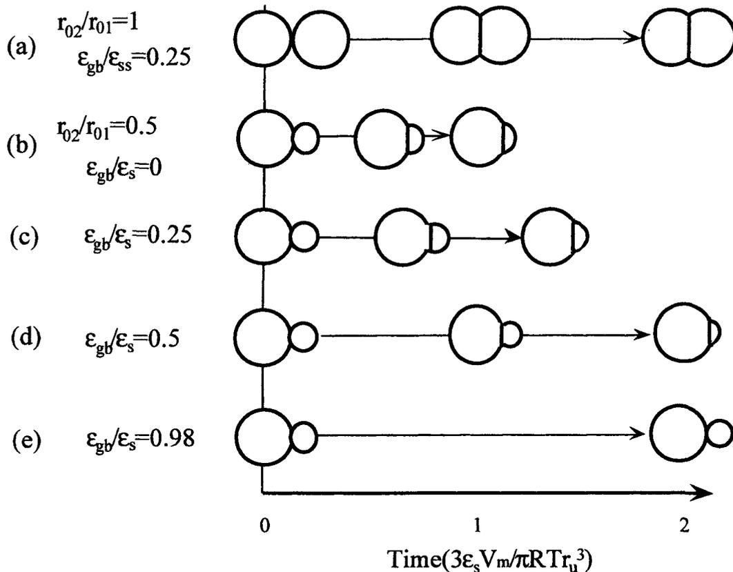
Fig.3 Sintering and grain growth behaviors of two grains as a function of grain size ratio  $r_{02}/r_{01}(=R_0)$  and ratio of grain boundary energy to surface energy,  $\alpha=\epsilon_{gb}/\epsilon_s$ .
