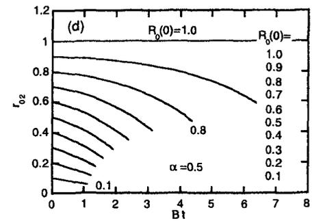
Fig.2 Changes in distance between grain center and grain boundary,  $X_{1,2}$ , and in grain radii,  $r_{01,02}$ , with sintering time  $Bt$ .  $B$  is normalizing factor,  $\epsilon_s D_x V_m / RT r_u^3$ , where  $r_u$  is unit of radius.
