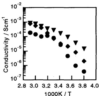
Fig. 4 Temperature dependence of conductivity for PAN-based electrolytes.
