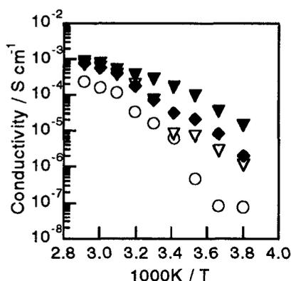
Fig. 2 Temperature dependence of conductivity for PAN-based electrolytes. (○): (PAN)<sub>20</sub>(LiClO<sub>4</sub>)<sub>4</sub>(PC)<sub>4</sub>
