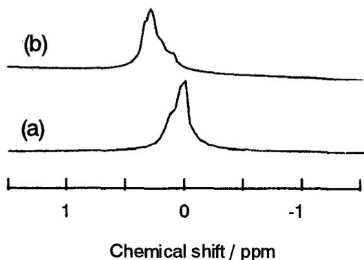
Fig. 5 <sup>7</sup>Li NMR spectra of PAN-based electrolytes at 50 °C.
