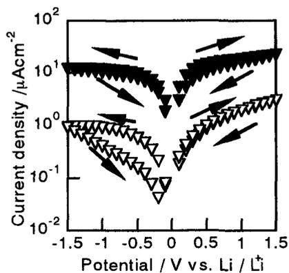
Fig. 6 Polarization curves of lithium electrode in PAN-based electrolytes.
