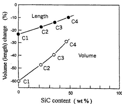
Fig.7 Relation between volume (length) change of the specimens carbonized (sintered) at 650 °C and SiC content.
