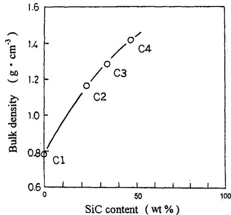
Fig.8 Relation between bulk density of the specimens carbonized (sintered) at 650 °C and SiC content.
