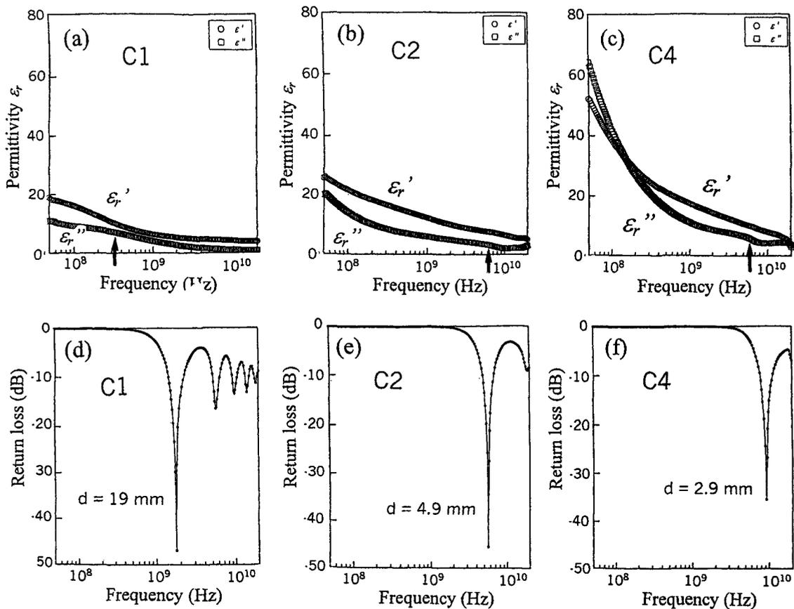
Fig.4 Frequency dependence of permittivities ( $\epsilon_r'$  and  $\epsilon_r''$ ) and wave absorption characteristics of the specimens carbonized (sintered) at 650°C. The value of d in the figure denotes the thickness needed for the peak absorption.
