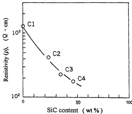
Fig.6 Relation between electrical resistivity of the specimens carbonized (sintered) at 650 °C and SiC content.
