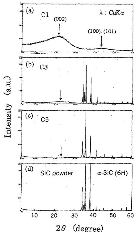
Fig.2 X-ray powder diffraction patterns of the specimens carbonized (sintered) at 650 °C and the starting SiC powder.
