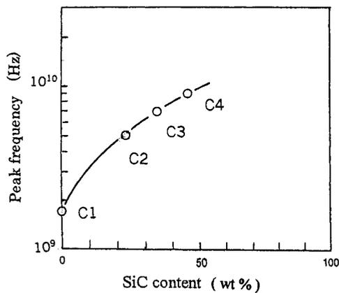
Fig.5 Relation between peak frequency of wave absorption and SiC content.
