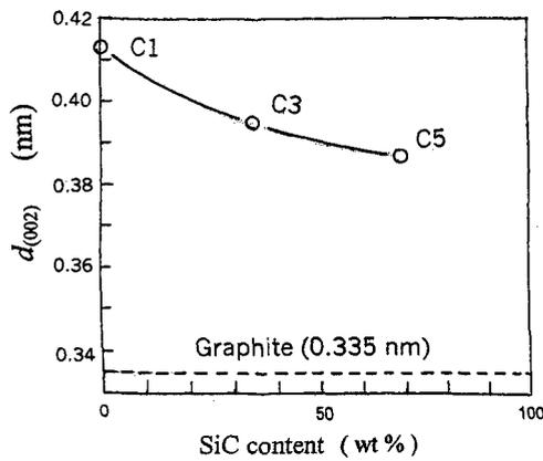
Fig.3 Change in lattice parameter ( $d_{002}$ ) of woodceramics matrix in the specimens carbonized (sintered) at 650 °C with increasing SiC content.
