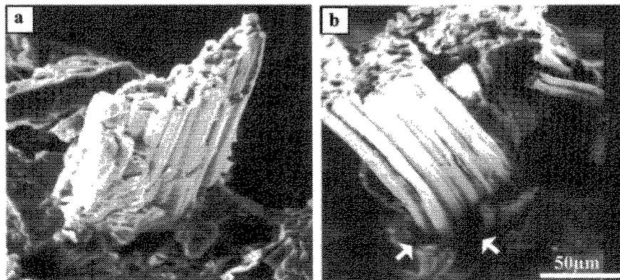
Fig. 6 Typical SEM photographs of the fracture surface for composite specimens containing 55% fiber area fraction, manufactured with (a) virgin PP and (b) recycled PP (molded at 175°C and formed under 10 MPa). Arrows indicate a gap between the interface.
