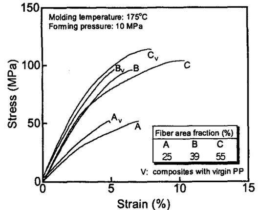
Fig. 1 Nominal stress-strain curves of composites with recycled PP matrix.
