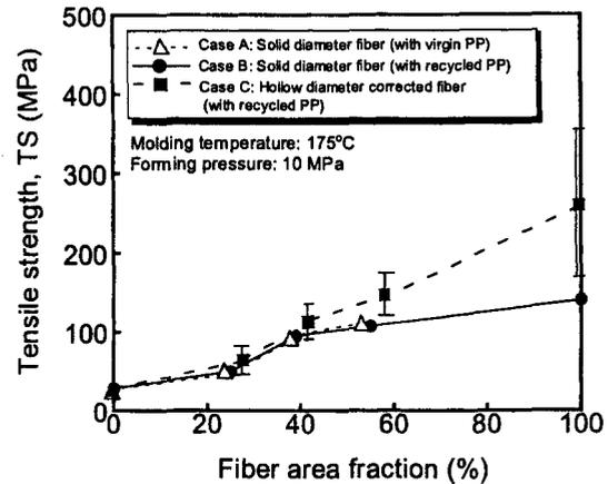
Fig. 2 Dependence of tensile strength on fiber area fraction.
