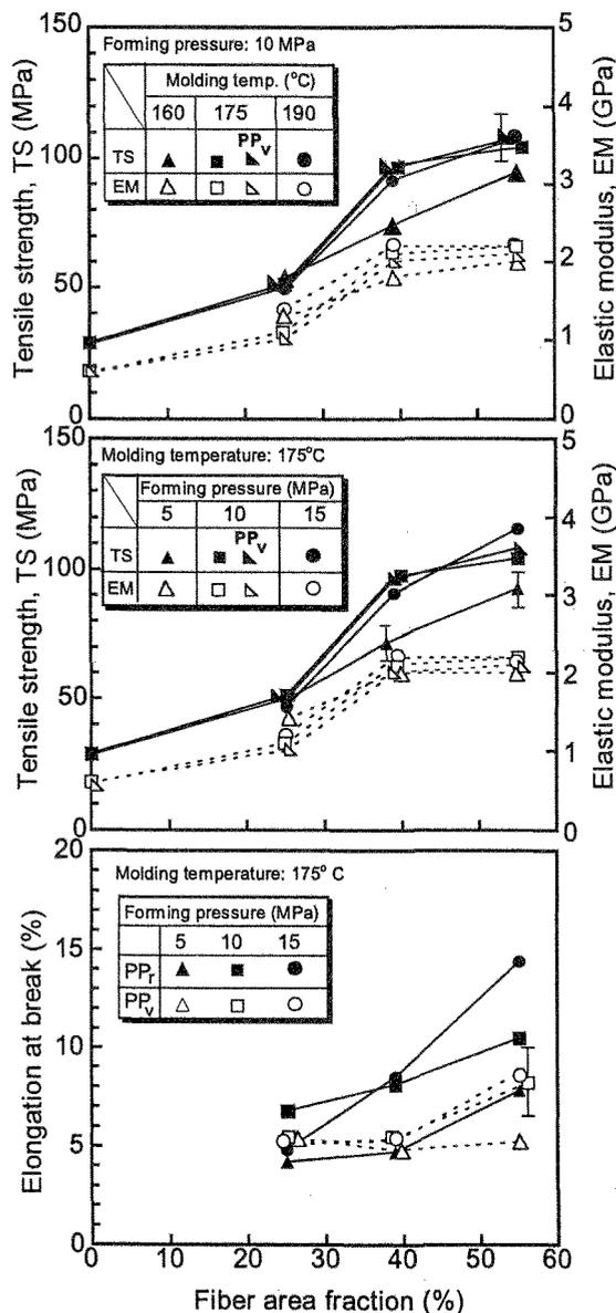
Fig. 3 Effect of fiber area fraction on tensile properties of composites with recycled PP matrix. PP<sub>v</sub> and PP<sub>r</sub> indicate composites manufactured with virgin PP and recycled PP, respectively.
