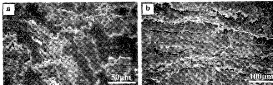
Fig. 5 SEM photographs of the cross-section of composite specimens (a) with virgin PP and (b) with recycled PP (55% fiber area fraction, molded at 175°C and formed under 10 MPa).
