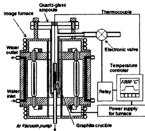
Fig. 1 Experimental configuration
