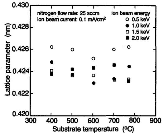
Fig. 1. The dependence of lattice parameters of TiN films on N ion-beam energy and substrate temperature.
