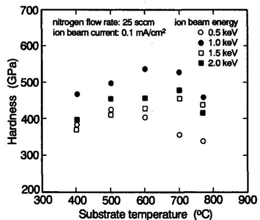
Fig. 2. The dependence of hardness  $H_f$  for TiN films on substrate temperature and N ion-beam energy.
