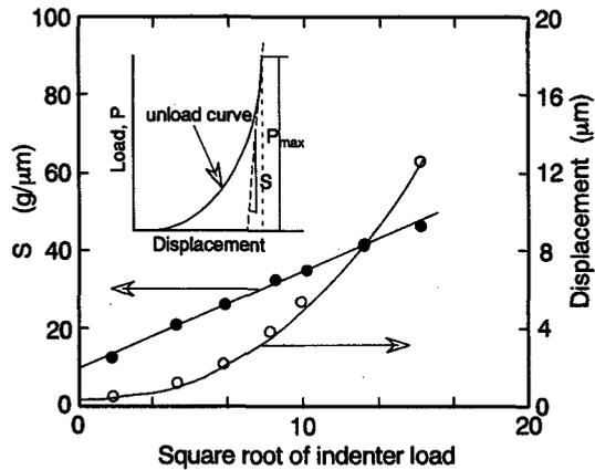
Fig. 3. Determination of S and A. The insert shows a load-displacement curve.
