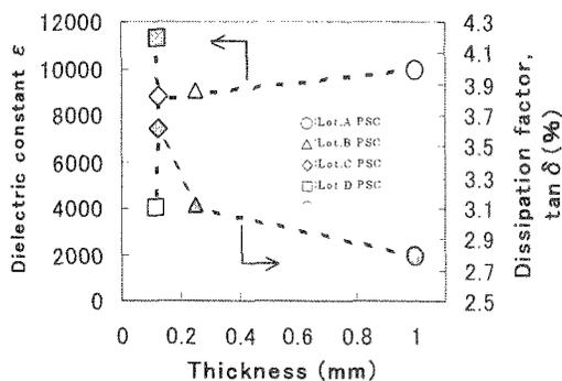
Fig.2 Dielectric constant  $\epsilon$  and dissipation factors  $\tan \delta$  of plate PSC oscillators before poling
