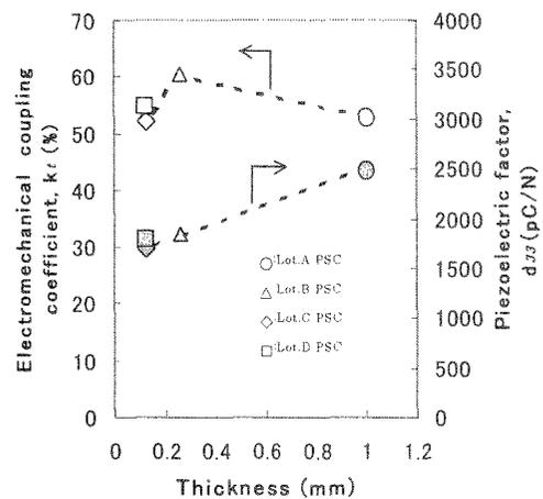
Fig.4 Piezoelectric factor  $d_{33}$  and electro-mechanical coupling coefficient  $k_t$
