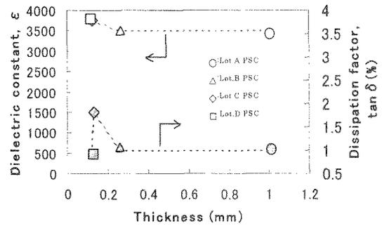
Fig.3 Dielectric constant  $\epsilon_{33}^T$  and dissipation factors  $\tan \delta$  of plate PSC oscillators after poling
