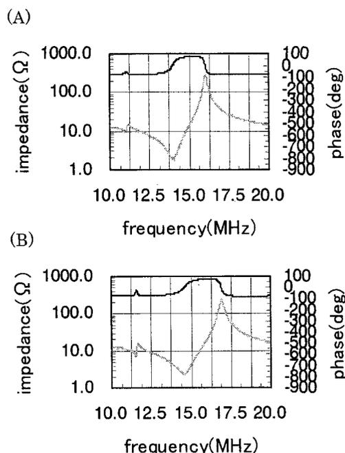
Fig.5 A typical frequency response and an impedance of a 0.128-mm-thick PSC oscillator (A) and a 0.120-mm-thick one (B)
