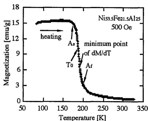
Fig. 2 Thermomagnetization curve on heating in a magnetic field of 500 Oe for Type II  $\text{Ni}_{53.5}\text{Fe}_{21.5}\text{Al}_{25}$  alloy.
