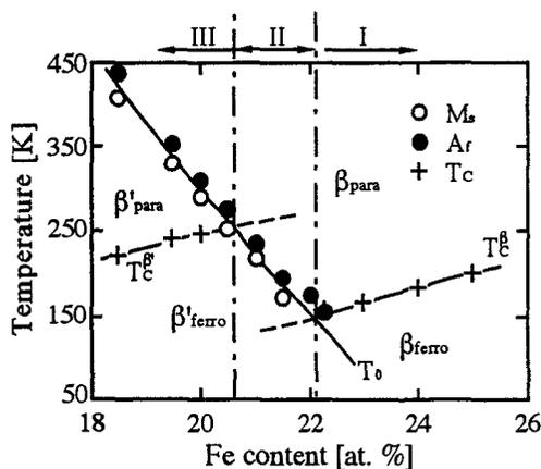
Fig. 1 Composition dependence of the Curie temperature  $T_c$ , the martensitic start  $M_s$  and the austenitic finish  $A_f$  temperatures, and the equilibrium temperature  $T_0 = (M_s + A_f)/2$  in  $\text{Ni}_{75-x}\text{Fe}_x\text{Al}_{25}$  alloys.
