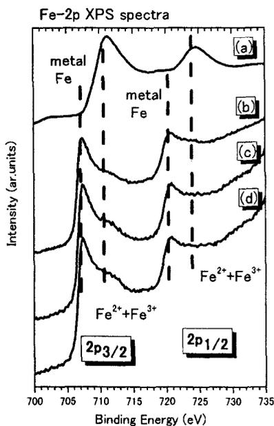
Fig.2 Fe 2p XPS spectra for (a)  $Fe_3O_4$  surface, (b) after Al overlayer, (c) post  $O_2$  exposure at  $5 \times 10^3$  Pa for 0.5h, and (d) post  $O_2$  exposure at  $5 \times 10^3$  Pa for 9.5h.
