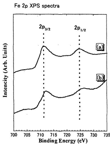
Fig.3 Fe 2p XPS spectra for Fe<sub>3</sub>O<sub>4</sub> surface before (a) and after (b) MgO (3 nm) layer deposition in 3x10<sup>-3</sup> Pa O<sub>2</sub>.
