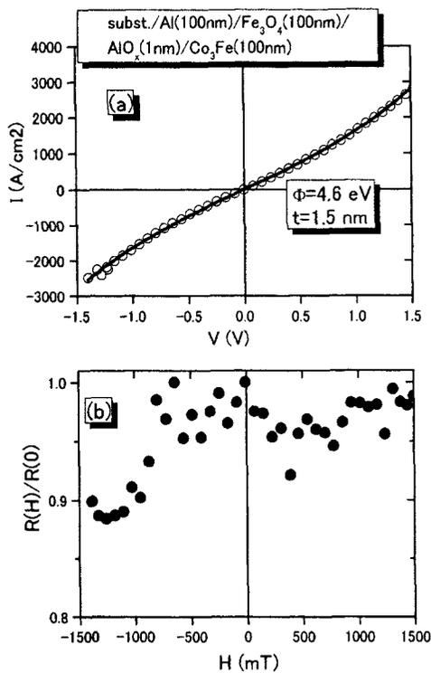
Fig.1 I-V curve (a) and MR result (b) for an aluminium oxide barrier sample. The solid line in (a) is a fitting result using Simons' equation.
