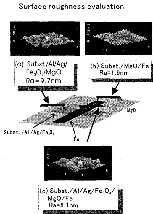
Fig.4 Various surface morphologies and average roughness (Ra) measured by a contact mode AFM. 1.5x1.5 mm area is scanned for a subst./Al(1 nm)/Ag(100 nm)/Fe<sub>3</sub>O<sub>4</sub>(50 nm)/MgO(5 nm)/Fe(50 nm) sample.
