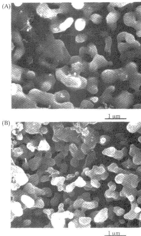
Fig.2 SEM photographs of monolithic sintered hydroxyapatites. (A) the *in-situ* process through pressureless sintering method with 10 T at 1373 K and (B) normal sintering process under 0 T at 1373 K.
