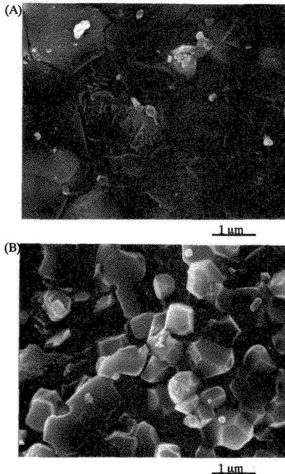
Fig.3 SEM photographs of sintered hydroxyapatite with  $\text{Na}_2\text{HPO}_4$ . (A) the *in-situ* process through pressureless sintering method with 10 T at 1373 K and (B) normal sintering process under 0 T at 1373 K.
