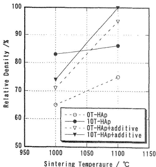
Fig.1 Relative density of monolithic hydroxyapatite and hydroxyapatite with disodium hydrogenphosphate as an additive.
