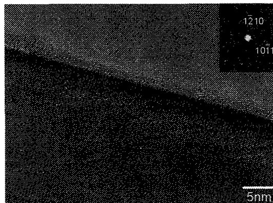
Fig. 4 HRTEM image and diffraction pattern of a B_{12.0}C_{3.0} thin film.
