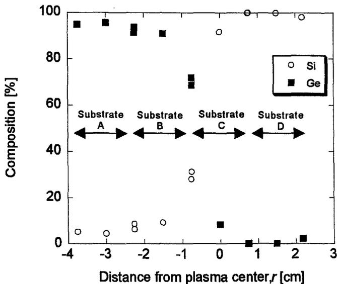
Fig. 5 Composition variation in  $\text{Si}_{1-x}\text{Ge}_x$  thin films measured by EDX. Positions of Substrates A-D are also shown.
