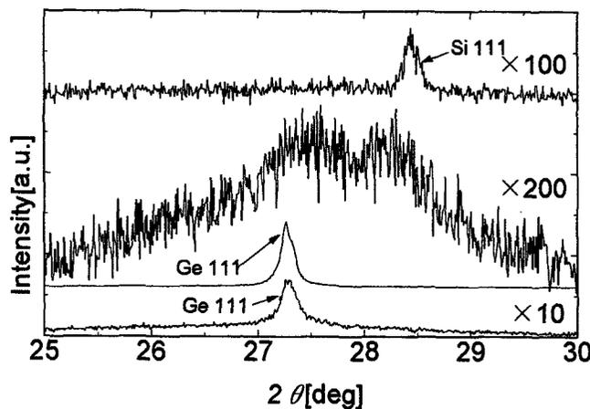
Fig. 4 XRD patterns for  $\text{Si}_{1-x}\text{Ge}_x$  thin film on Substrates A-D.
