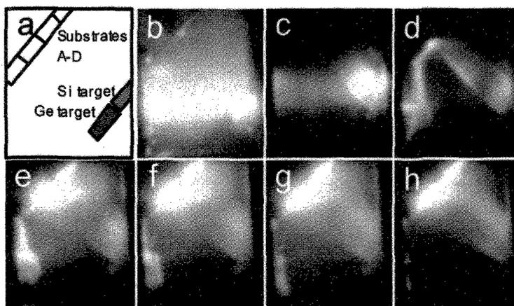
Fig. 3 (a): schematic diagram of Si and Ge targets and Substrates A-D, (b)-(h): high-speed photographs of ablation plasma from the Si-Ge hybrid target.
