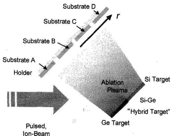
Fig. 2 Schematic diagram of position of Substrates A – D for preparation of compositionally gradient  $\text{Si}_{1-x}\text{Ge}_x$  thin film.
