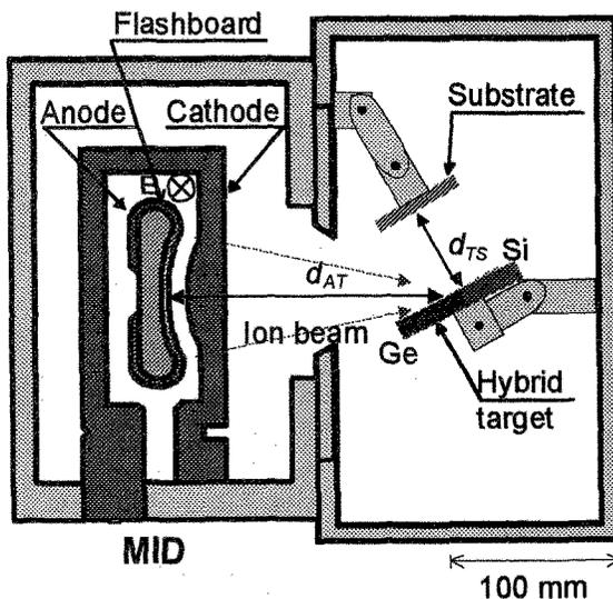
Fig. 1 Schematic diagram of ion-beam diode and thin film preparation chambers for production of compositionally gradient  $\text{Si}_{1-x}\text{Ge}_x$  thin films.
