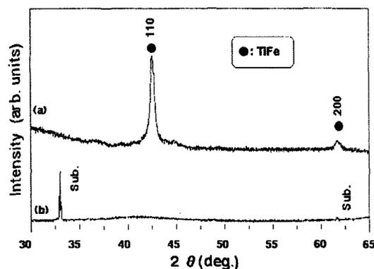
Fig. 3 XRD patterns of the thin films deposited by using Ti-40 at.%Fe target at  $d_{AT} = 180$  mm and  $d_{TS} = 90$  mm on (a) glass substrate, (b) Si(100) substrate.
