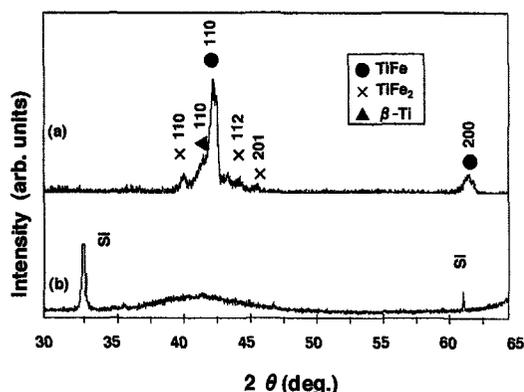
Fig. 2 XRD patterns of the thin films deposited by Ti-50 at.%Fe target at  $d_{AT} = 170$  mm and  $d_{TS} = 90$  mm on (a) glass substrate, (b) Si(100) substrate.
