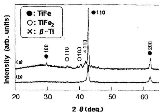
Fig. 4 XRD patterns of the thin films (a) before and (b) after hydrogenation treatments.
