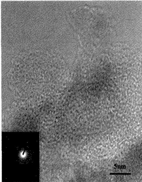
Fig. 2 HRTEM image and diffraction pattern of soot prepared by PWD using copper electrodes.
