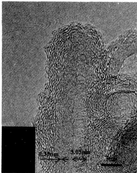
Fig. 3 HRTEM image and diffraction pattern of soot prepared by PWD using stainless steel electrodes.
