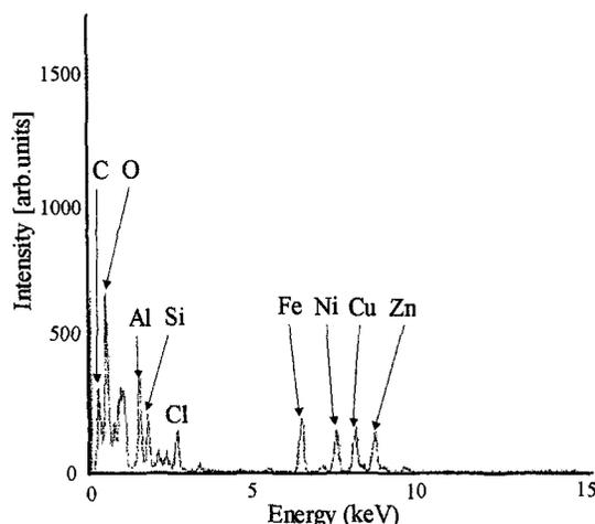
Fig. 6 EDX data of soot prepared by PWD and with the use of copper electrodes.
