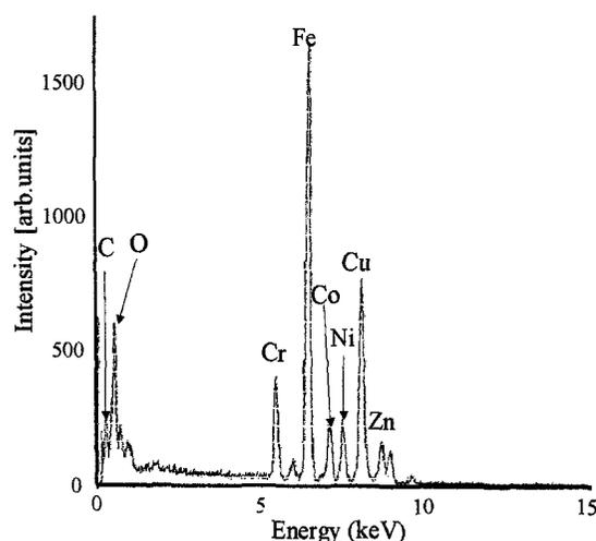
Fig. 5 EDX data of soot prepared by PWD and with the use of stainless steel electrodes.
