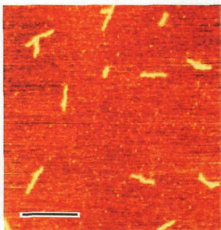
**Figure 1.** AFM image of *Samia cynthia ricini* fibroin sample, cast over mica immediately after filtering. Tapping mode, mica substrate, scale bar : 500nm.
