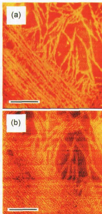
**Figure 3.** AFM image of *Samia cynthia ricini* fibroin sample, cast over mica 24 hours after filtering. (a): topographic image (b): phase image. tapping mode, mica substrate, scale bar : 500nm.
