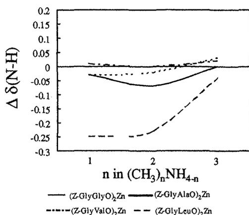
Fig. IV Chemical shift changes of  $\delta(\text{N-H})$  in the mixture of  $(Z\text{-GlyGlyO})_2\text{Zn}$ ,  $(Z\text{-GlyAlaO})_2\text{Zn}$ ,  $(Z\text{-GlyValO})_2\text{Zn}$  and  $(Z\text{-GlyLeuO})_2\text{Zn}$  with  $(\text{CH}_3)_n\text{NH}_{4-n}$ , where  $n=1,2$  and 3.
