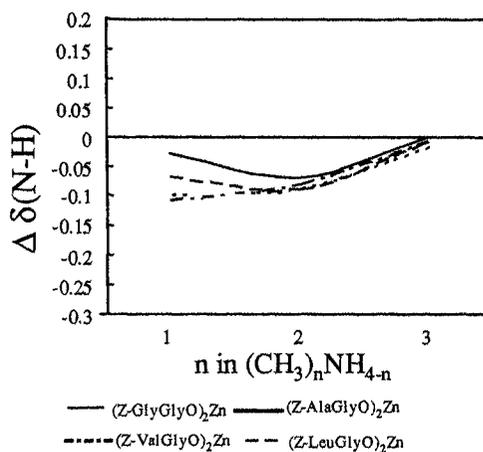
Fig. IV Chemical shift changes of  $\delta(\text{N-H})$  in the mixture of  $(Z\text{-GlyGlyO})_2\text{Zn}$ ,  $(Z\text{-AlaGlyO})_2\text{Zn}$ ,  $(Z\text{-ValGlyO})_2\text{Zn}$  and  $(Z\text{-LeuGlyO})_2\text{Zn}$  with  $(\text{CH}_3)_n\text{NH}_{4-n}$ ,  $n=1,2$  and 3.
