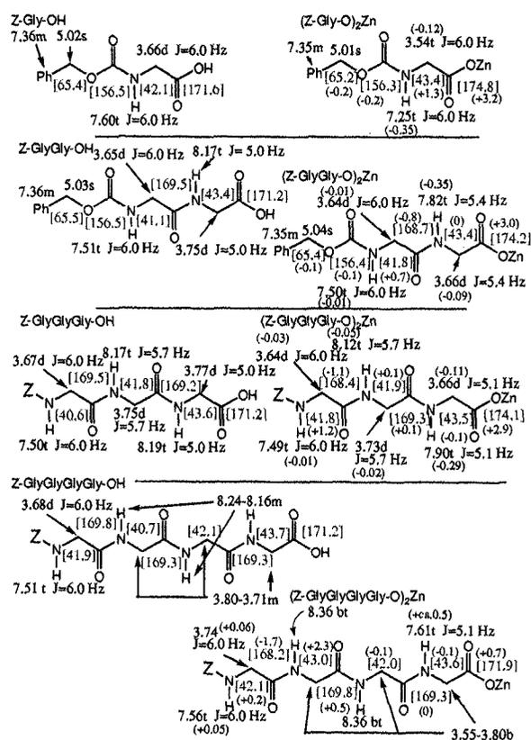
Figure 1 NMR assignments of ligands and Zn complexes. Chemical shifts  $\delta$  of <sup>1</sup>H and <sup>13</sup>C are displayed around the molecular formulae and the differences of the chemical shifts between the ligands and complexes are also represented in parentheses.
