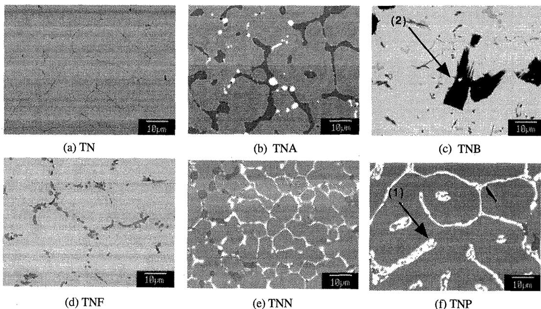
Fig.1 Microstructures of specimens before test.
