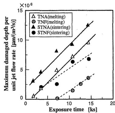
Fig.7 Comparison of melting method with sintering method.
