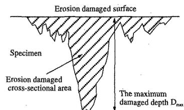
Fig.3 Determination of the damaged cross-sectional area and the maximum damaged depth.
