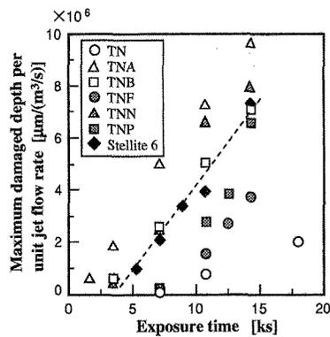
Fig.5 Maximum damaged depth per unit jet flow rate in Ti-Ni base alloys and Co-based alloy.
