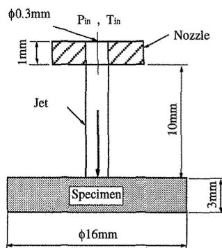
Fig.2 Schematic flow diagram.
