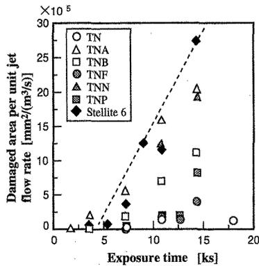
Fig.4 Damaged area per unit jet flow rate in Ti-Ni base alloys and Co-based alloy.
