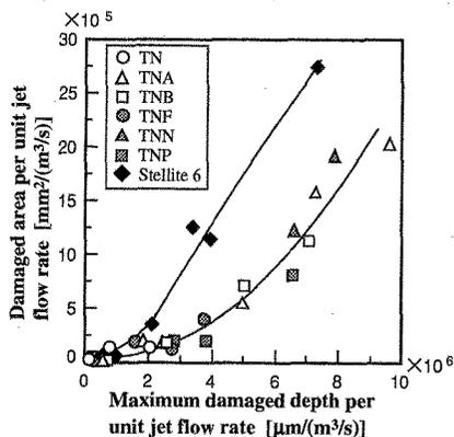
Fig.9 Relationship between damaged area and the maximum damaged depth.
