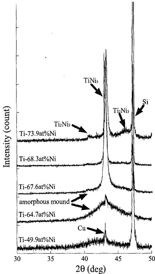
Fig.1 The XRD patterns for Ti-49.9~73.9at%Ni as-sputtered thin films
