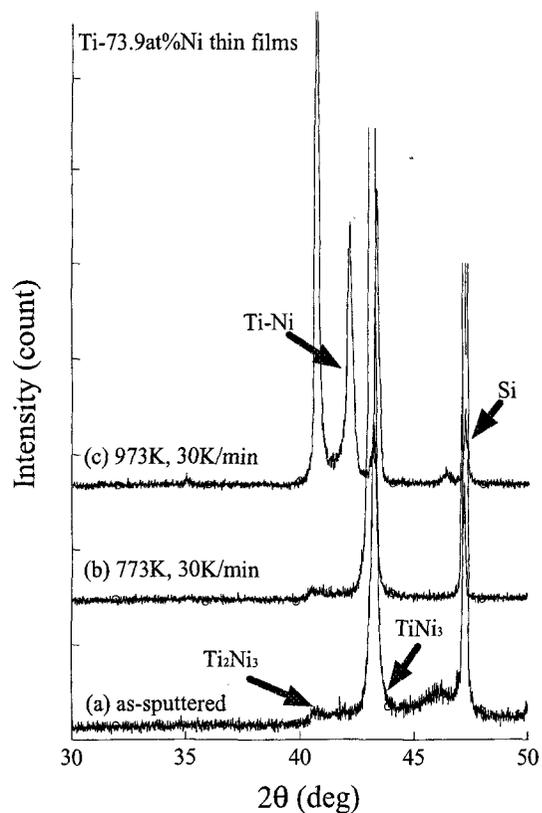
Fig.6 XRD patterns of Ti-73.9at%Ni thin films: (a) as-sputtered, (b) heated up to 773K and (c) heated up to 973K at 30K/min.
