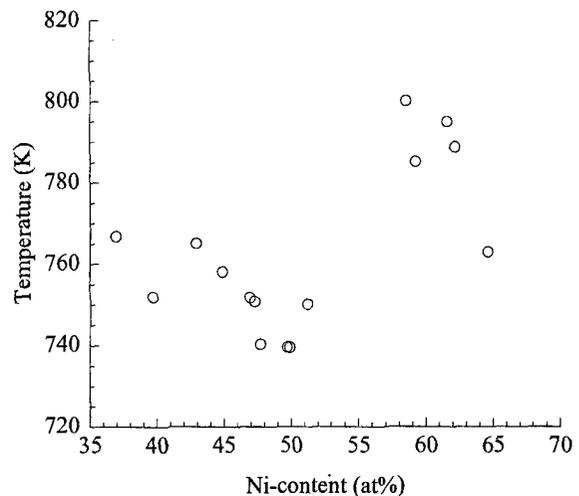
Fig.3 Relationship between the DSC peak temperature of crystallization obtained at 10K/min and Ni-content
