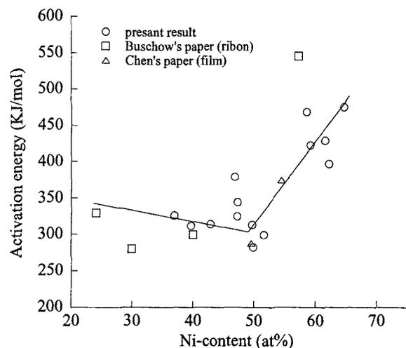
Fig.4 Relationship between the activation energy for crystallization and Ni-content
