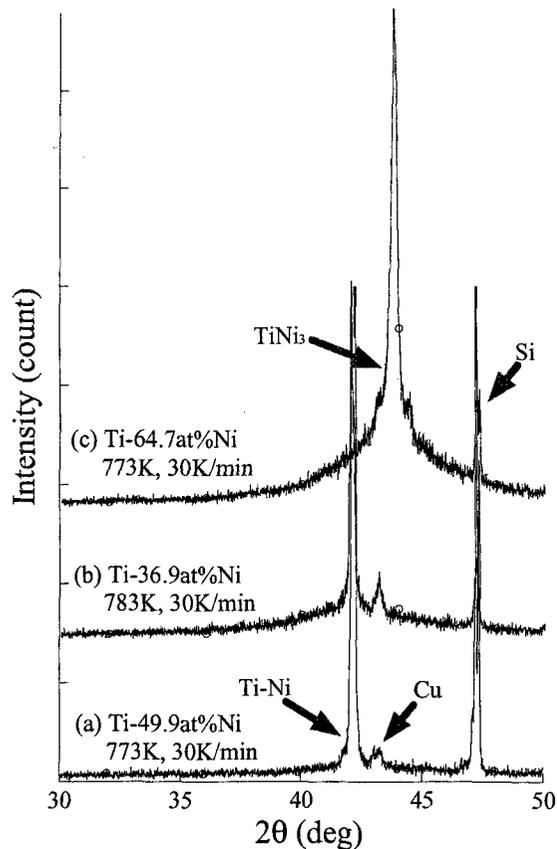
Fig.5 XRD patterns of (a) Ti-49.9at%Ni, (b) Ti-36.9at%Ni and (c) Ti-64.7at%Ni thin films.
