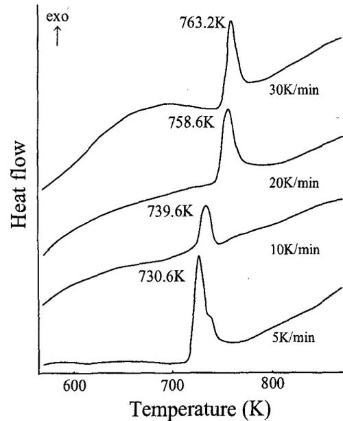
Fig.2 DSC curves with different heating rates for the Ti-49.9at%Ni thin film.
