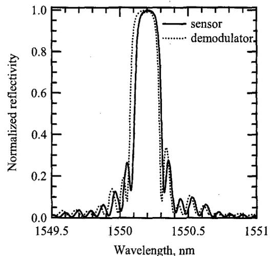
Fig. 3 Reflective characteristics of FBGs employed.
