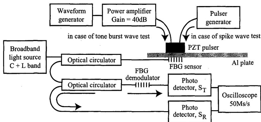
Fig. 1 Experimental setup of AE measurement using FBGs.
