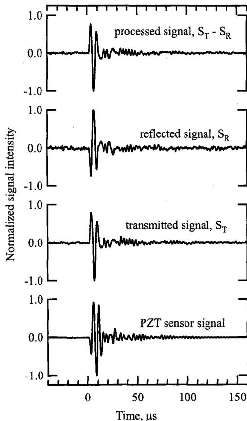
Fig. 4 Response of FBG and PZT sensors to spike wave.
