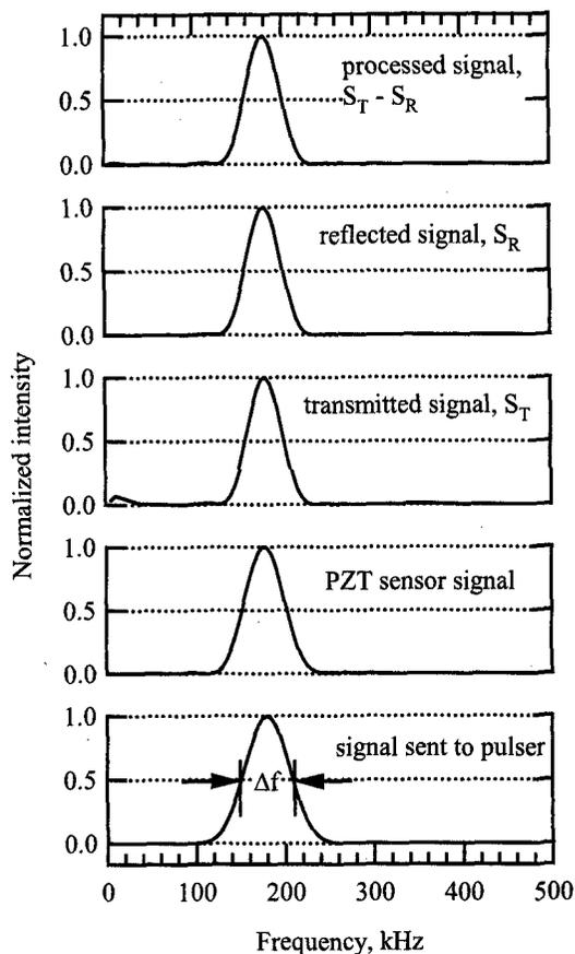
Fig. 7 Frequency analysis on signals responded to tone burst wave.
