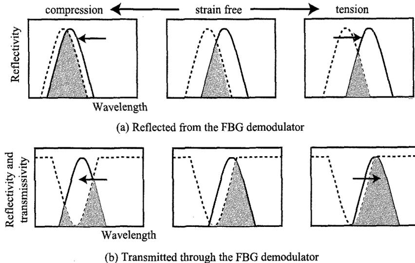
Fig. 2 Schematics illustrating change in intensity of the demodulated light with varying strain.
