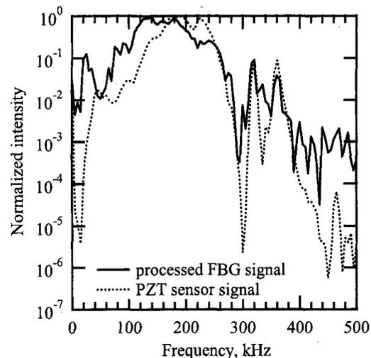
Fig. 5 Frequency analysis on signals responded to spike wave.
