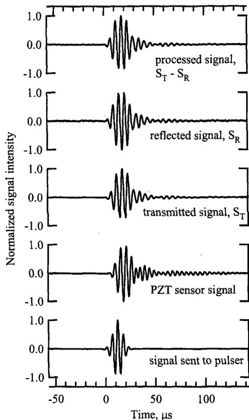
Fig. 6 Response of FBG and PZT sensors to tone burst wave.
