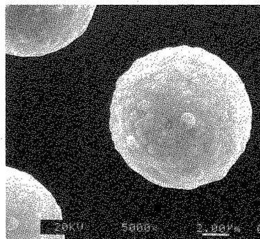
Fig.2 SEM image of polystyrene particles coated with Ni-P alloy layer.
