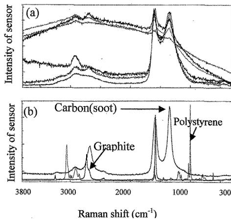
Fig.5 Laser Raman spectra of the materials inside cell walls.
