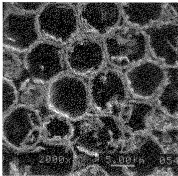
Fig. 4. Cross-section of the metallic closed cellular material.
