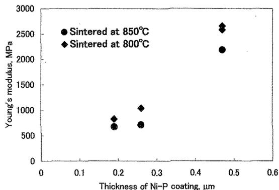
Fig. 8. Relationship between thickness of the cell walls and Young's Modulus of closed cellular materials.
