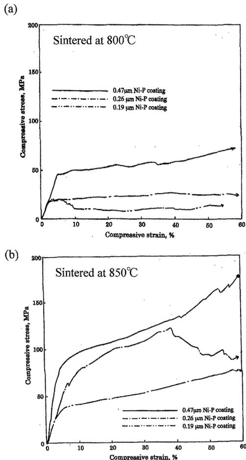
Fig. 6. Compressive stress-strain curve for metallic closed cellular materials; (a) sintered at 800°C and (b) sintered at 850°C.
