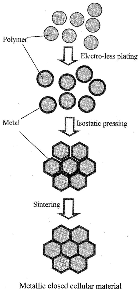
Fig. 1 Flow diagram of metallic closed cellular material fabricating process
