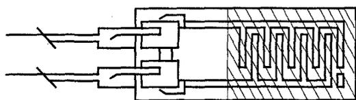
Fig. 2 Schematic diagram of humidity sensor with comb-shaped electrodes
