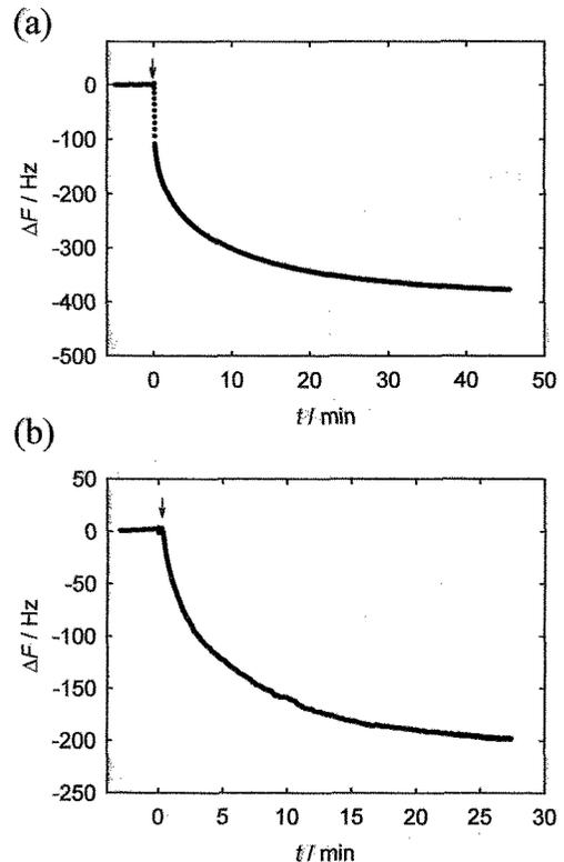
Fig. 2. Typical time course of frequency change of collagen deposited QCM in response to the addition of dsDNA (a) and ssDNA (b). 100  $\mu\text{l}$  of DNA solution was added at the time indicated the arrow.
