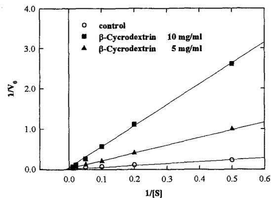
Fig. 3. The Lineweaver-Burk plot with the addition of  $\beta$ -CD (10 or 5 mg/ml) to the synthetic substrate-thrombin system.
