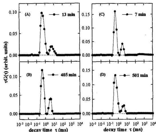
Fig. 2. Time evolution of the decay time distribution function  $\tau G(\tau)$  in the presence of 18.2 mg/ml  $\beta$ -CD-S (A),(B) and 0.1 mg/ml heparin (C),(D). (A) and (C) are at the initial stage of the reaction, and (B) and (D) are at several hours after the reaction start.
