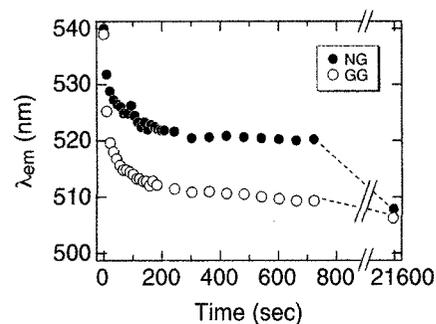
**Figure 2.** Temporal change in  $\lambda_{em}$  of dansyl probe for NG and GG after T-jump from 10°C to 35°C.
