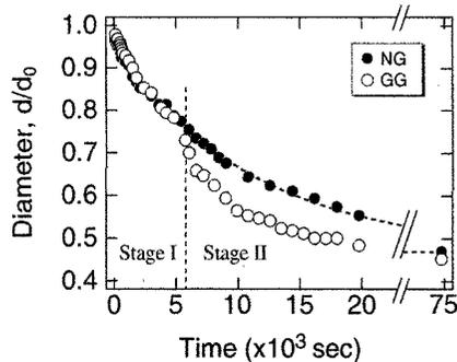
**Figure 1.** Variation of  $d/d_0$  of the NG and GG after T-jump from 10°C to 35°C. The line is the fit with eq. 4.
