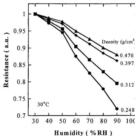
Fig.3 Humidity dependence of the electrical resistance for WCMs with different density.
