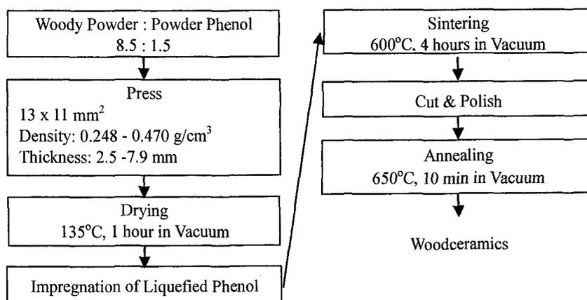
Fig.1 Fabrication process for woodceramics
