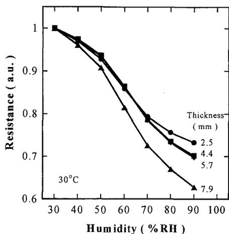
Fig.5 Humidity dependence of the resistance for WCMs with various thicknesses.
