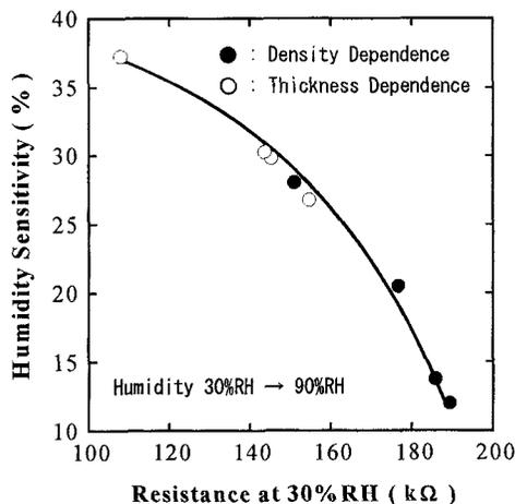
Fig.4 Relationship between the sensitivity to humidity and the resistance at humidity of 30%RH.
