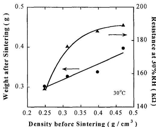
Fig.2 Relationship between the weight and the electrical resistance for WCMs after sintering and the density before sintering.
