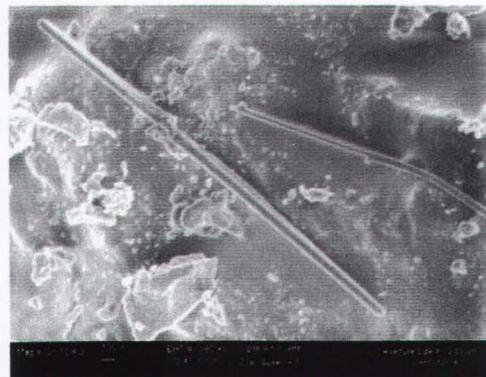
Fig. 1 SEM photograph of cedar-based woodceramics.
