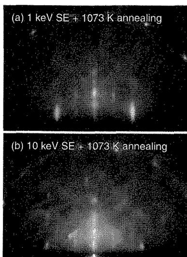
Fig. 5 RHEED patterns of Si (100) substrate after (a) 1 keV SE and post-irradiation annealing and (b) 10 keV SE and post-irradiation annealing. Similar pattern was observed for 3 keV SE and post-irradiation annealing.
