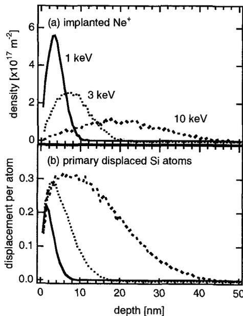
Fig. 1 Calculated depth distribution of (a) implanted Ne<sup>+</sup> and (b) primary displaced Si atoms. Incident ion energies are 1 keV (solid line), 3 keV (dotted line), and 10 keV (dashed line).
