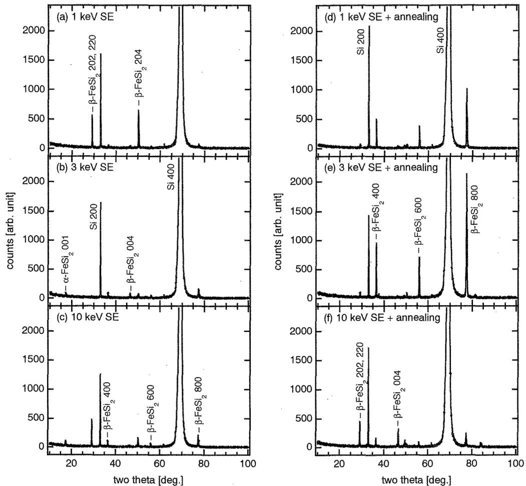
Fig. 2 The XRD spectra of  $\text{FeSi}_2$  films formed with various surface treatments. (a) - (c): SE only and (d) - (f): SE, followed by annealing at 1073 K for 30 minutes.
