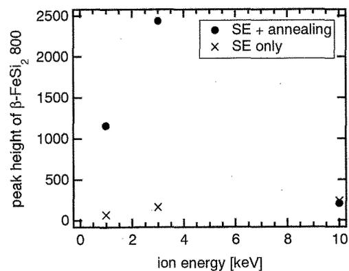
Fig. 3 The peak height of  $\beta\text{-FeSi}_2$  800 reflection in all XRD spectra shown in Fig. 2.
