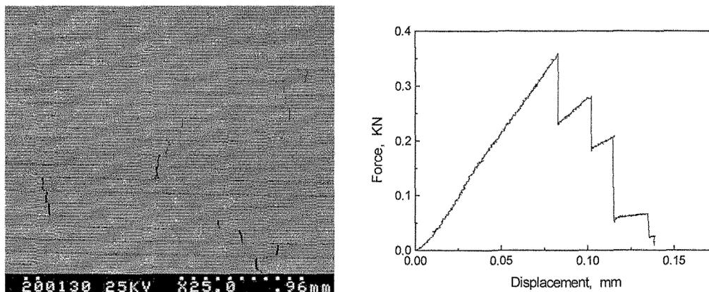
Fig.5 Fracture path and corresponding load-displacement response in SiC/BN-Al<sub>2</sub>O<sub>3</sub>-SiC laminated composite
