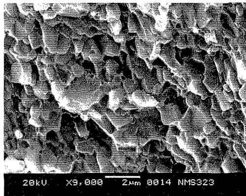
Fig.1 SEM micrograph of SiC matrix block material on fracture surface.
