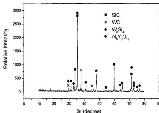
Fig.2 X-ray diffraction pattern of SiC/W composite
