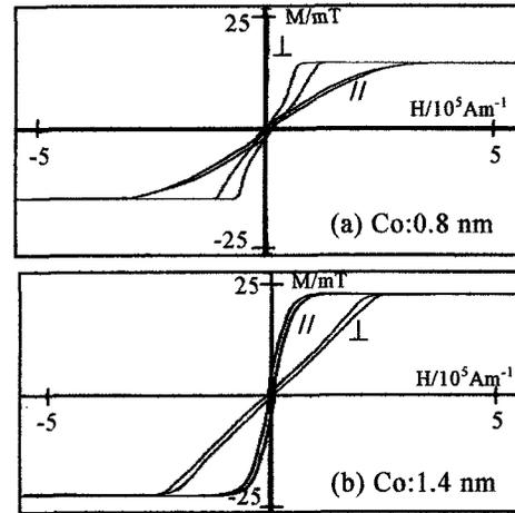
**Fig 1.** Magnetization curve with Co layer thickness.
