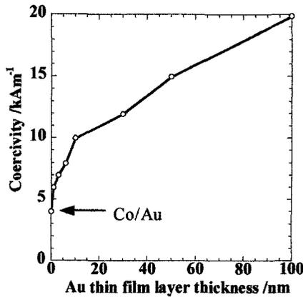
Fig 2. Coercivity with the Au thin film layers.
