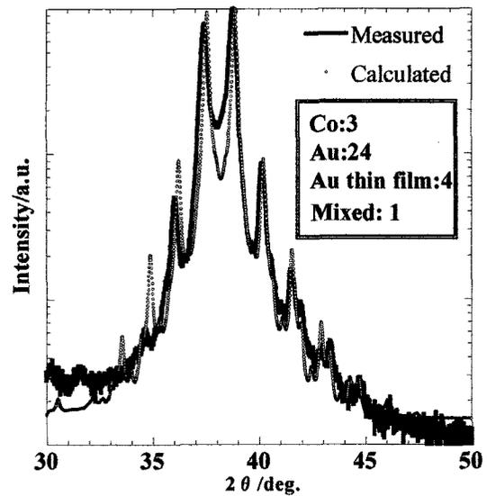
Fig 6. Profile fitting by the extended 3-step model in the high angle region. (473 K, 1 h-annealing)
