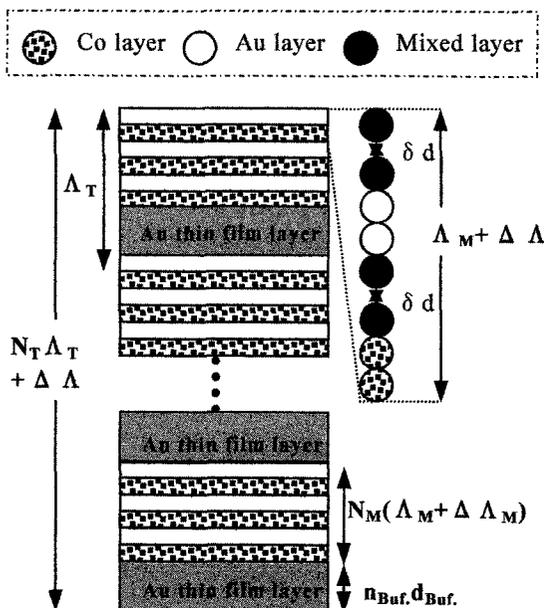
Fig 5. Schematic view of the extended 3-step model.
