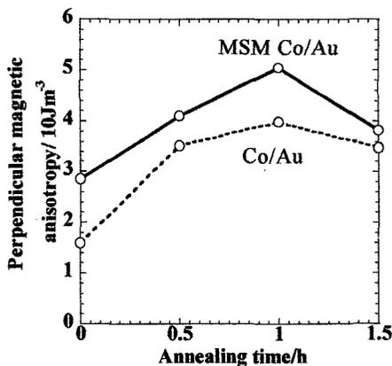
Fig 4. Perpendicular magnetic anisotropy with annealing.
