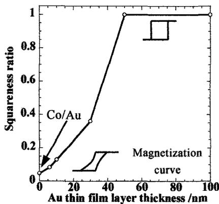
Fig 3. Squareness ratio with the Au thin film layers.
