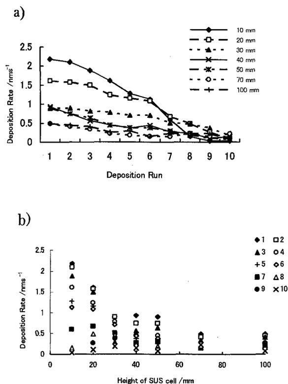
Figures 2 (a) The dependence of deposition rate on the deposition run with SUS cells which have different height. The height of SUS cell was varied from 10 to 100 mm. (b) The dependence of deposition rate on the height of SUS cell.
