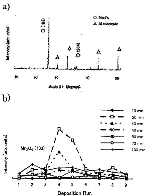
Fig. 3 (a) A XRD pattern of a film prepared with SUS cell height of 20 mm. (b) The variation of XRD peak strength with increasing deposition run. The parameter is the height of SUS cell.
