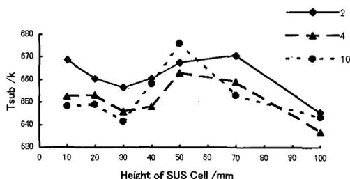
Fig. 4 The dependence of substrate temperature ( $T_{\text{sub}}$ ) on the height of SUS cell.
