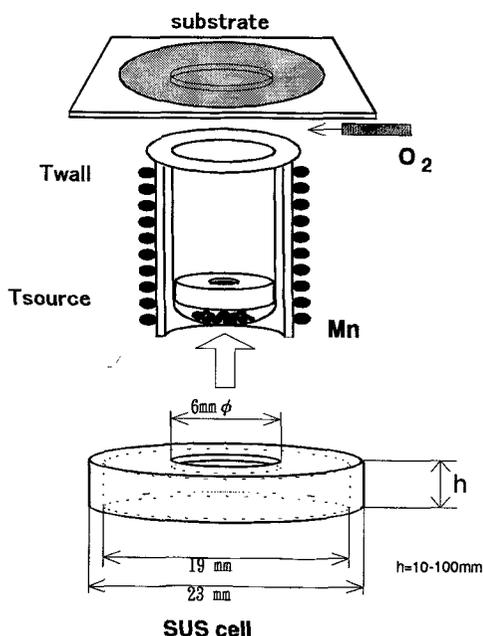
Fig. 1 Schematic of a SUS cell. The stainless steel (SUS) cell with a hole is set in the bottom of the crucible.
