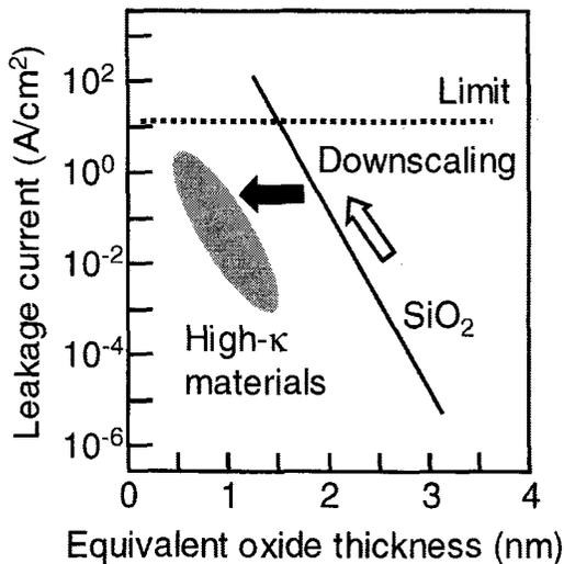
Fig. 2. Physical limits of  $\text{SiO}_2$  systems.
