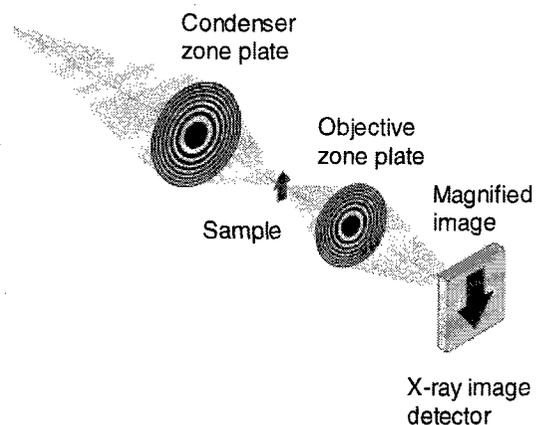
Fig. 3. Schematic diagram of transmission X-ray microscope. The X-rays are collected by the condenser zone plate and projected onto a sample. The image of this region is magnified by the objective zone plate and projected onto the X-ray image detector.
