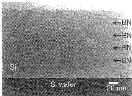
Figure 8. Cross-sectional TEM image of multiple BN delta layers. Thickness of BN layer: 0.1 nm. Thickness of Si layer: 18 nm.
