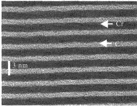
Figure 5. Cross-sectional TEM image of Cr/C multilayer
