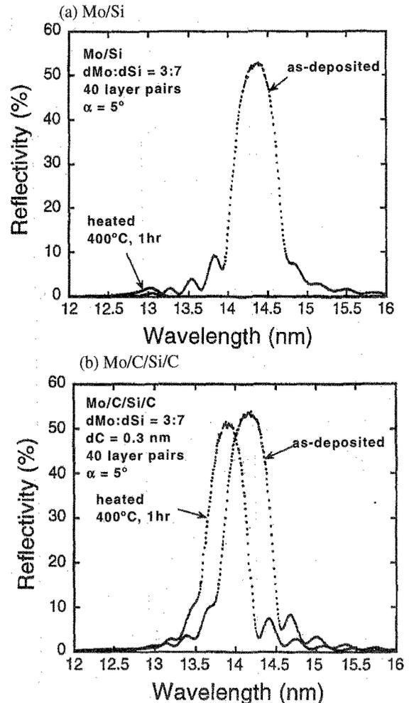
Figure 4. Measured reflectivities of as-deposited and 400°C-annealed (a) Mo/Si multilayers and (b) Mo/C/Si/C multilayers at an incident angle of 85°. Each has 40 pairs of layers. The period is 7.2 nm for the Mo/Si multilayer and 7.3 nm for the Mo/C/Si/C multilayers.
