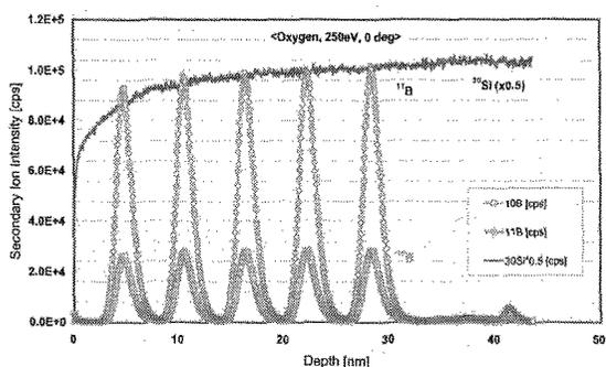
Figure 9. High resolution SIMS depth profile of multiple short-period BN delta layers. Thickness of BN layer: 0.05 nm. Thickness of Si layer: 5 nm. The data was obtained using 250 eV  $O_2^+$  at  $30^\circ$  incidence.
