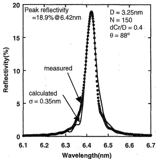
Figure 6. Measured and calculated (fitted) reflectivity of Cr/C multilayer.
