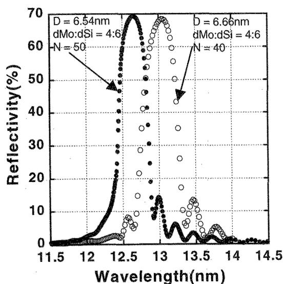
Figure 1. Measured reflectivities of Mo/Si multilayers at an incident angle of 88°. Closed circles: 69.3% @  $\lambda = 12.6$  nm. Open circles: 68.4% @  $\lambda = 13$  nm.
