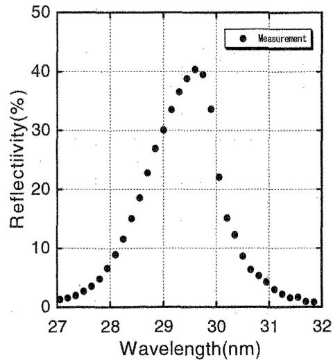
Figure 7. Measured reflectivity of Mg/SiC multilayer for an incident angle of  $88^\circ$ .
