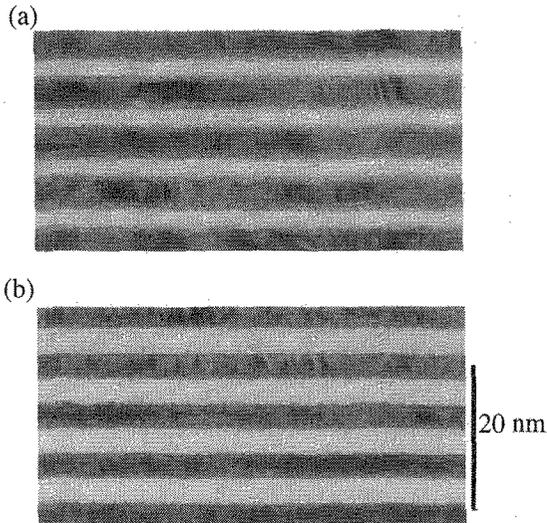
Figure 2. Cross-sectional TEM image of (a) Mo/Si multilayer and (b) Mo/C/Si/C multilayer.
