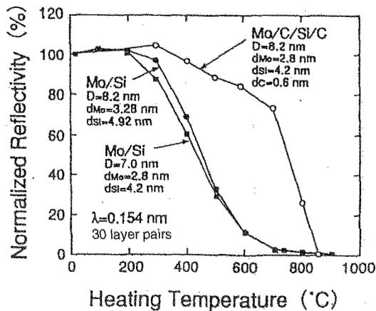
Figure 3. Relationship between normalized Cu-K $\alpha$  first-order Bragg-peak reflectivity of Mo/Si and Mo/C/Si/C multilayers and heating resistance.
