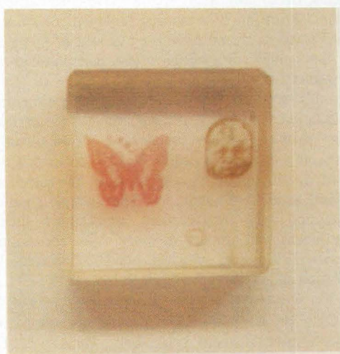
Figure 3. Photograph of images drawn inside the glass sample by using a femtosecond laser: gray-colored image (after femtosecond laser irradiation) and red-colored butterfly (after femtosecond laser irradiation and further heat treatment at 550°C for 1 hour).
