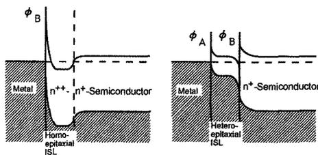
Fig. 2. Energy band diagrams of metal/semiconductor interfaces with highly doped ISL (a) and low energy barrier ISL (b).
