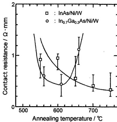
Fig. 3. Contact resistances of the  $\text{In}_{0.7}\text{Ga}_{0.3}\text{As}/\text{Ni}/\text{W}$  contact (shown by circles) annealed at various temperatures by RTA.
