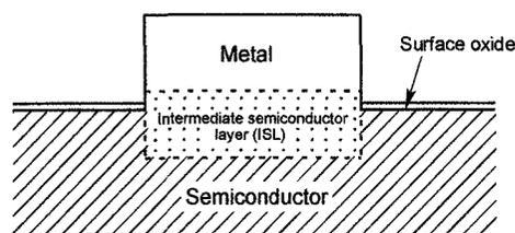
Fig. 1 . Cross-section of metal/semiconductor interface with intermediate semiconductor layer (ISL).
