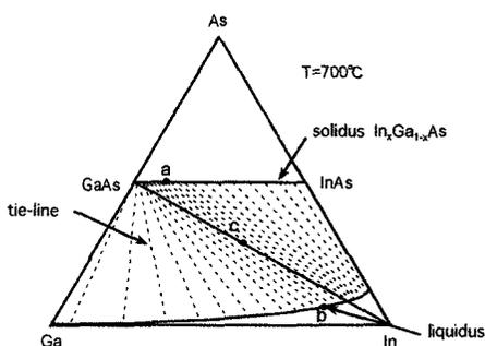
Fig. 4. Ternary InGaAs phase diagram calculated at 700°C.
