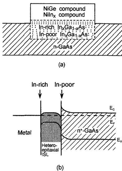
Fig. 7. Microstructure at the metal/GaAs interface of NiInGe contact which provided low  $R_C$  (a) and the corresponding band diagram(b).
