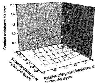
Fig. 6. Contact resistances as functions of In concentration and volume fraction of  $\text{In}_x\text{Ga}_{1-x}\text{As}$  layers .
