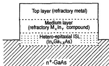
Fig. 5. Cross-section of ideal In-based ohmic contact.
