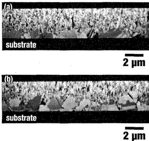
Figure 2 Cross-sectional SIM image of the sputtered Cu film on the  $\text{Si}_3\text{N}_4$  substrate, annealed at 298 K for (a) 4h or (b) 72h
