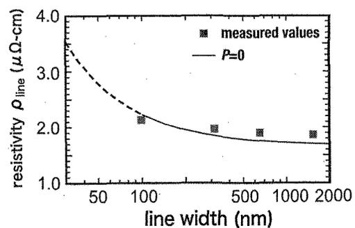
Figure 4 Measured resistivity of single-crystal Cu interconnects as a function of line width
