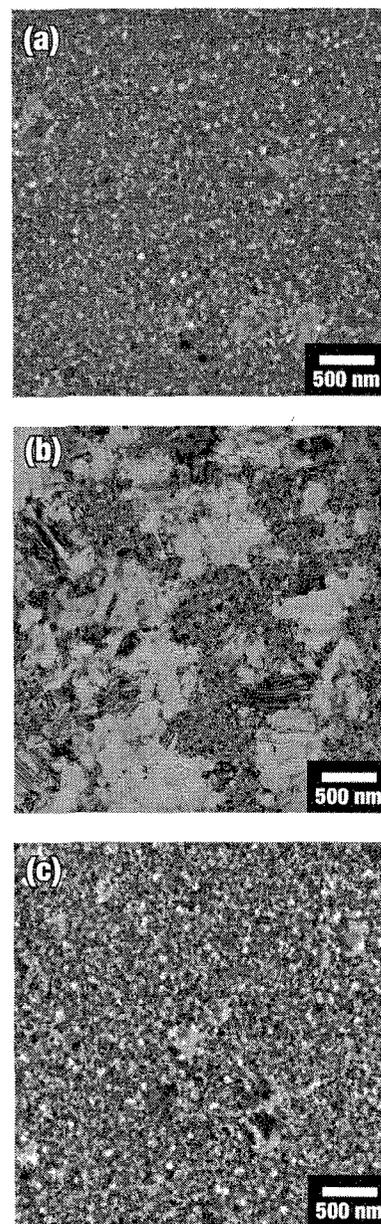
Figure 1 Plan-view TEM image of the 100 nm-thick sputtered Cu film deposited on the rocksalt substrate, annealed at 298 K for (a) 3 h, (b) 264 h, or (c) 192 h without substrate.
