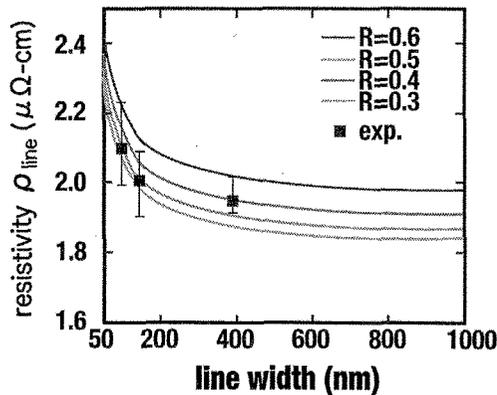
Figure 5 Resistivity of poly-crystal Cu interconnects which have mean grain size of 700 nm as a function of line width.
