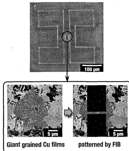
Figure 3 Interconnect pattern for resistivity measurement, which was patterned in a giant grained Cu films by FIB technique.
