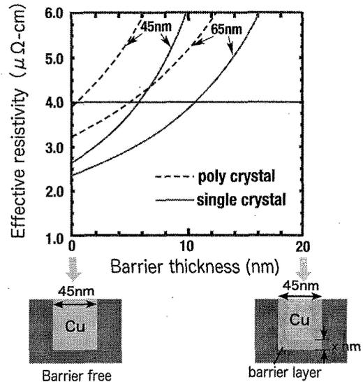
Figure 6 Effective resistivity in Cu damascene interconnects with line width of 65 nm and 45 nm as a function of barrier thickness.
