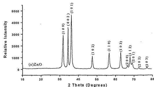
Fig. 2 The XRD patterns of as-prepared product
