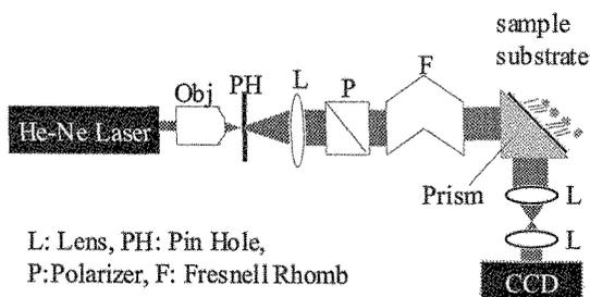
Fig.1 Schematic for SPR imaging experiment
