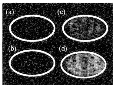
Fig. 4 SPR images of DNA monolayers. Incident angle was set the SPR angle of bare Au thin film. (a) BD monolayer. (b) BD-T1 monolayer. (c) Colloidal Au attached BD monolayer. (d) Colloidal Au attached BD-T1 monolayer.
