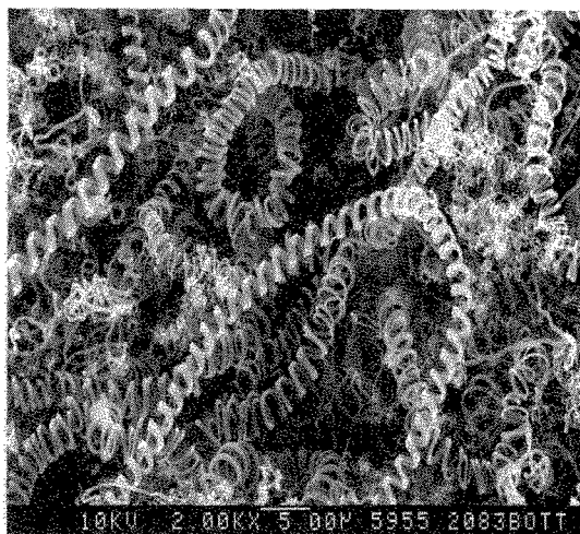
Fig. 8. Super-elastic carbon microcoils obtained by stopping and re-starting at 770^\circ\text{C} .
