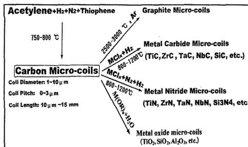
Fig. 12. Modification process of carbon coils.
