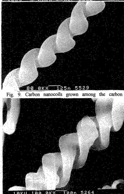
Fig. 10. A carbon nanocoil with dumbbell-type cross-section.
