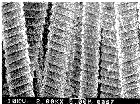
Fig. 1. Representative regular carbon microcoils with constant coil diameter and coil pitches along the coil.
