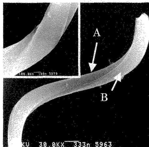
Fig. 6. The carbon coil with a very large coil pitch.
