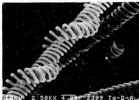
Fig. 4. The twined carbon microcoil with different coil length
