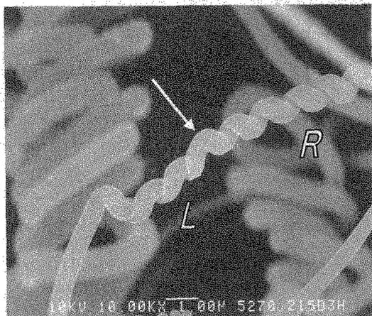
Fig. 10 Twisting carbon nanocoil with coiling chirality changed.
