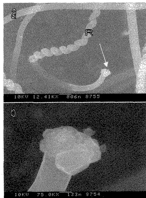
Fig. 9 Another growth tip of the twisting carbon nanocoil which is of one-directional growth.
