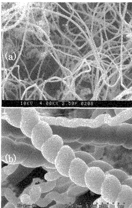
Fig. 2 Mass amount of twisting carbon nanocoils grown on the surface of thick carbon fibers.
