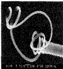
Fig. 7 A growth tip of a carbon microcoil.
