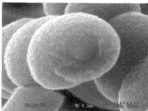
Fig. 3 Microstructure of the twisting carbon nanocoil.
