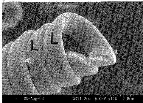
Fig. 6 Cross sections of a flat-fiber carbon microcoil.
