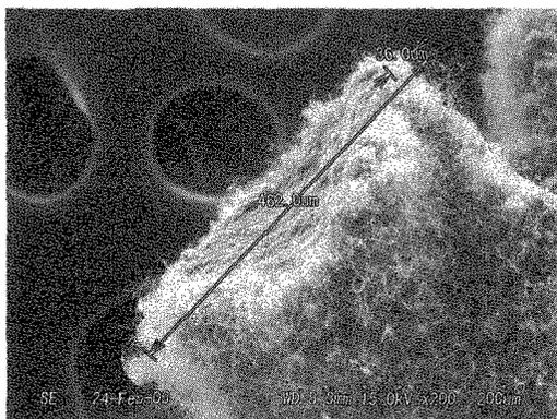
Fig. 1 Twisting carbon nanocoils grown on the surface of a thick carbon fiber.
