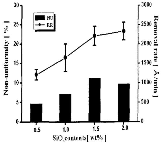
Fig. 5. Removal rates and non-uniformity as a function of SiO<sub>2</sub> contents in the 1 : 10 diluted silica slurry.
