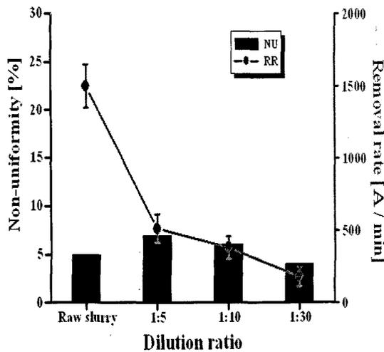
Fig. 4. Removal rates and non-uniformity as a function of dilution ratio.
