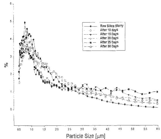
Fig. 2. Particle size analysis of original silica slurry in 30<sup>th</sup> days.
