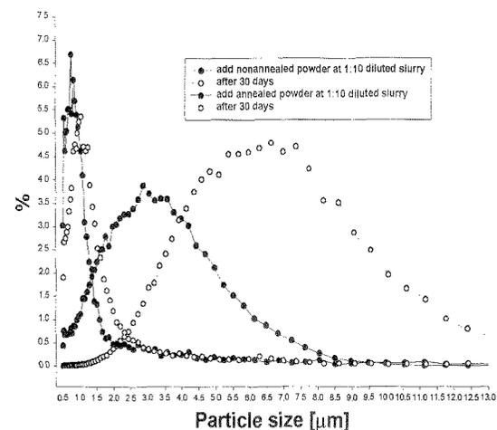
Fig. 3. Particle size analysis of MAS after 30 days.
