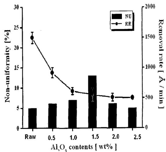
Fig. 6. Removal rate and non-uniformity as a function of Al<sub>2</sub>O<sub>3</sub> abrasive contents in the 1:10 diluted silica slurry.
