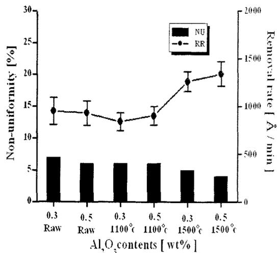
Fig. 7. Removal rate and non-uniformity as a function of annealed Al<sub>2</sub>O<sub>3</sub> abrasive contents in the 1:10 diluted slurry.
