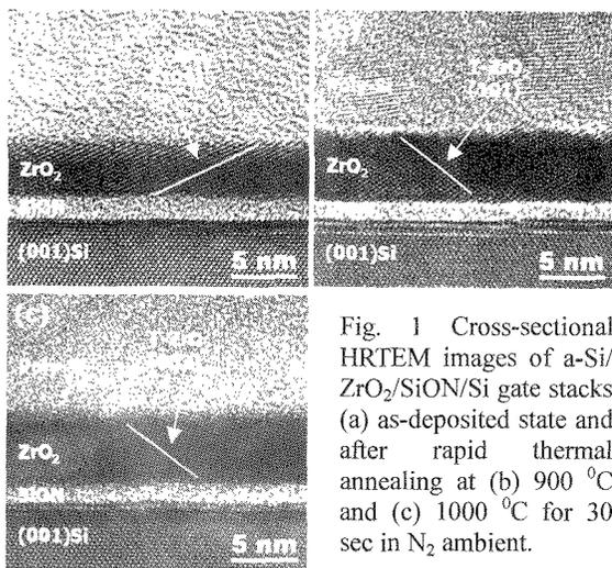
Fig. 1 Cross-sectional HRTEM images of a-Si/ZrO<sub>2</sub>/SiON/Si gate stacks (a) as-deposited state and after rapid thermal annealing at (b) 900 °C and (c) 1000 °C for 30 sec in N<sub>2</sub> ambient.
