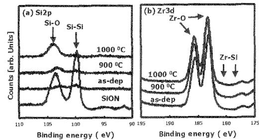
Fig. 2 The XPS analysis (a) before and (b) after rapid thermal annealing of the ZrO<sub>2</sub>/SiON/Si gate stack structure showing changes in the Si 2p and Zr 3d spectra. The bottom photoelectron spectra in (a) was obtained from the SiON/Si sample.
