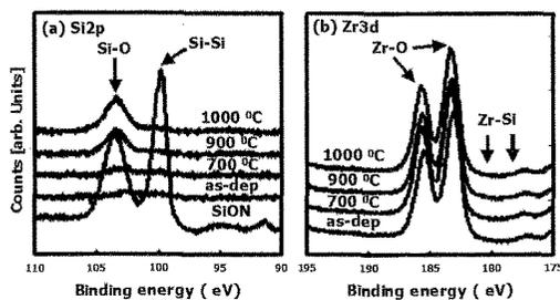
Fig. 4 The XPS analysis (a) before and (b) after rapid thermal annealing of the (Zr,Ti)O<sub>2</sub>/SiON/Si gate stack structure showing changes in the Si 2p and Zr 3d spectra.
