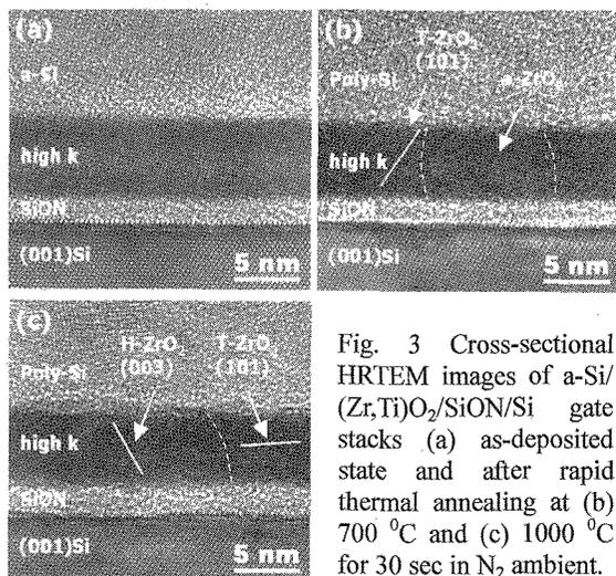
Fig. 3 Cross-sectional HRTEM images of a-Si/(Zr,Ti)O<sub>2</sub>/SiON/Si gate stacks (a) as-deposited state and after rapid thermal annealing at (b) 700 °C and (c) 1000 °C for 30 sec in N<sub>2</sub> ambient.
