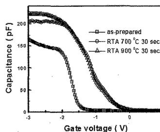
Fig. 5 High frequency (100 kHz) C-V characteristics of the Al/TaN/ZrO<sub>2</sub>/SiON/p-Si MIS capacitors after RTA in N<sub>2</sub> ambient for 30 sec at different temperatures.
