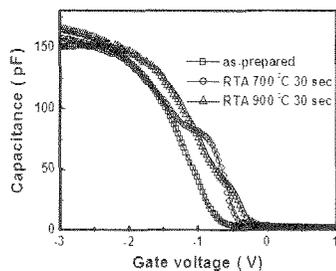
Fig. 6 High frequency (100 kHz) C-V characteristics of the Al/TaN/(Zr,Ti)O<sub>2</sub>/SiON/p-Si MIS capacitors after RTA in N<sub>2</sub> ambient for 30 sec at different temperatures.
