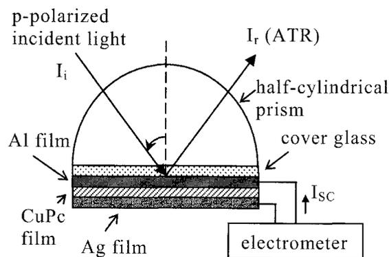
Fig. 2. Structure of the photoelectric cells fabricated in this work and arrangement for ATR and  $I_{sc}$  measurements based on the Kretschmann configuration.
