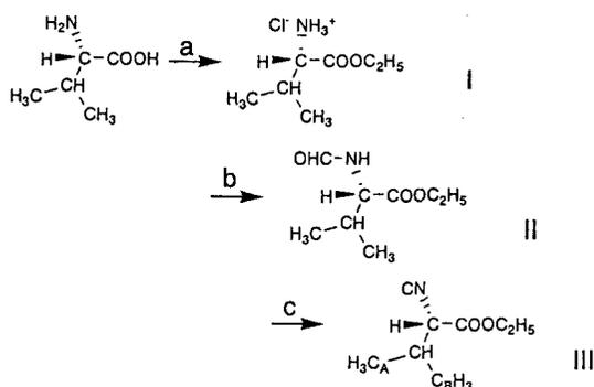
**Scheme 1.** Synthetic route of isocyanide monomer derived from L-valine. (a) ethanol,  $\text{SOCl}_2$ , r.t. (b) acetic formic anhydride in formic acid, r.t. (c) bis(trichloromethyl)carbonate, triethylamine in  $\text{CH}_2\text{Cl}_2$ ,  $-10^\circ\text{C}$ .
