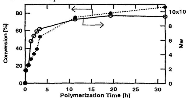
**Figure 1.** Time courses of the monomer conversion (dotted line) and the polymerization (solid line) of the isocyanide monomer III in methanol at room temperature.  $[\text{III}] = 1.0\text{ mol/l}$ .  $[\text{III}] / [\text{Ni(II)}] = 100$ . Both conversion and MW were determined by GPC (polystyrene standard).
