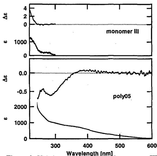
**Figure 2.** UV-vis and CD spectra (a) monomer III and (b) poly05 in  $\text{CHCl}_3$ .
