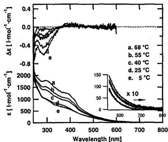
**Figure 3.** UV-vis and CD spectra of poly05, poly25, poly40, poly55, and poly68 in  $\text{CHCl}_3$ , which were obtained by polymerization at 5, 25, 40, 55, and 68 °C, respectively. The measurements were carried out at room temperature. The details on the isolation procedure and the sample preparation are described in the text.
